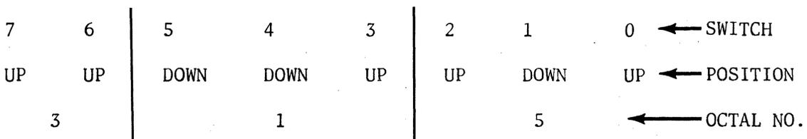
Note that switches 8 through 15 were not used. Switches 0 through 7 correspond to the switches labeled DATA on the front panel. A memory address would use all 16 switches.
