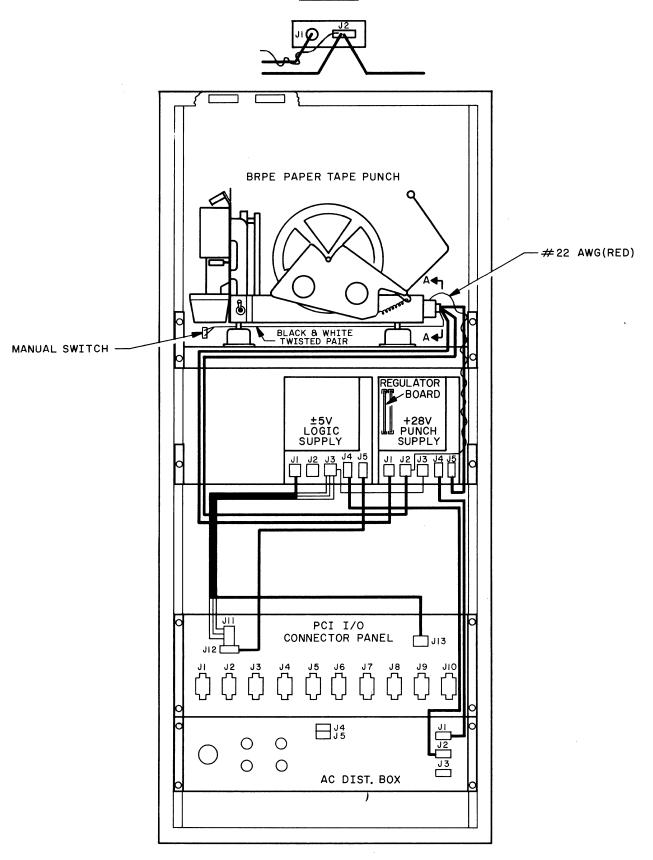
FIGURE 10-1 BRPE RACK CABLING
