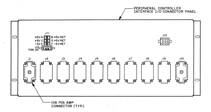
FIGURE 2-6 PCI I/O CONNECTOR PANEL
