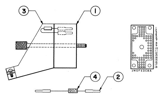
FIGURE 2-13 I/O TERMINATOR
