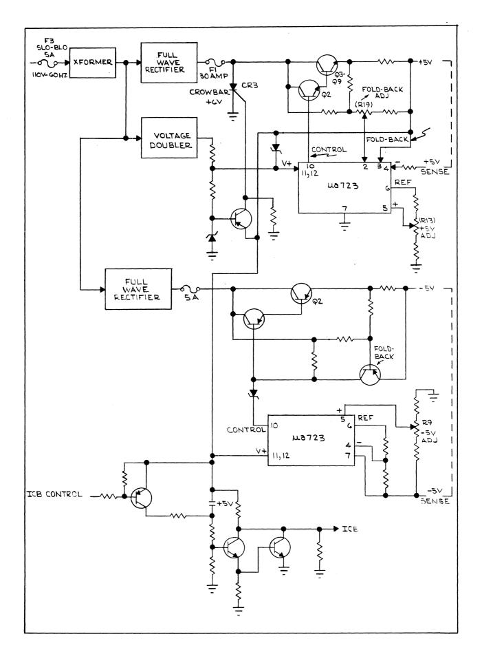
FIGURE 2-7 +5V POWER SUPPLY FUNCTIONAL DIAGRAM
