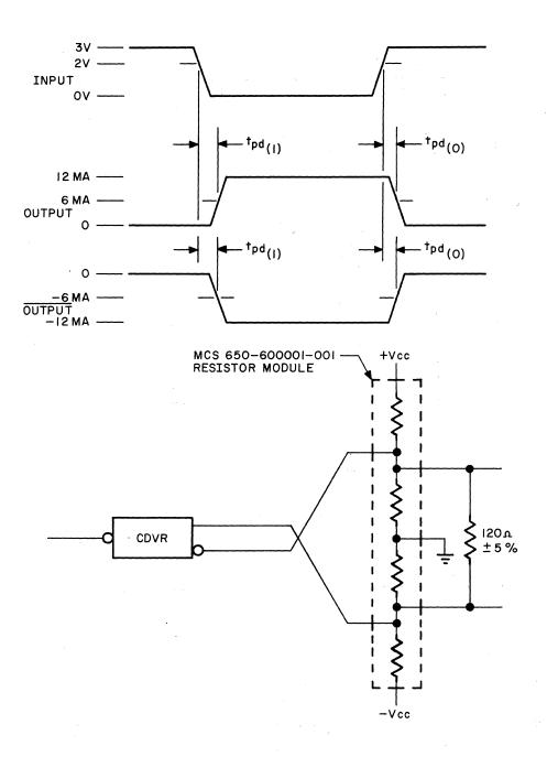
FIGURE 2-11 WAVE FORMS AND TERMINATION NETWORK
