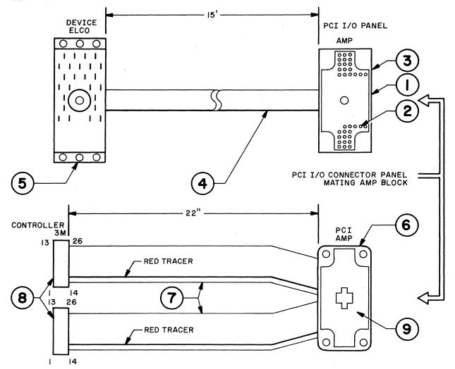
FIGURE 6-2 CARD READER I/O CABLING
