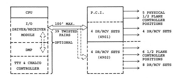
FIGURE 2-2 PCI/CPU INTERFACE FUNCTIONAL BLOCK DIAGRAM Standard plane numbering and coordinates, including the 26 pin 3M I/O connector locations are illustrated in Figure 2-3.
