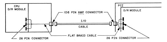
FIGURE 2-5 I/O BUS INTERCONNECTION DIAGRAM
