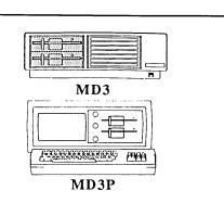
The only substantial difference between the MD3 and MD3P is that the MD3P has the monitor built-in (making it portable, in theory). They both have two double-sided floppy disk drives.
