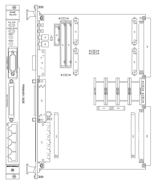
Figure 2-1. MVME162LX Switch, Header, Connector, Fuse, and LED Locations
