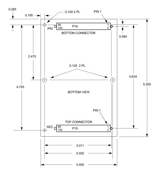
Figure D-2. Mezzanine Board Dimensions (SRAM and ECC DRAM)
