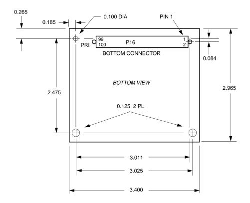
Figure D-1. Mezzanine Board Dimensions (Parity DRAM)
