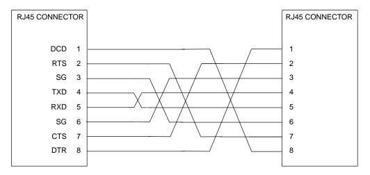
Figure A-4. Typical RJ45 Serial Cable
