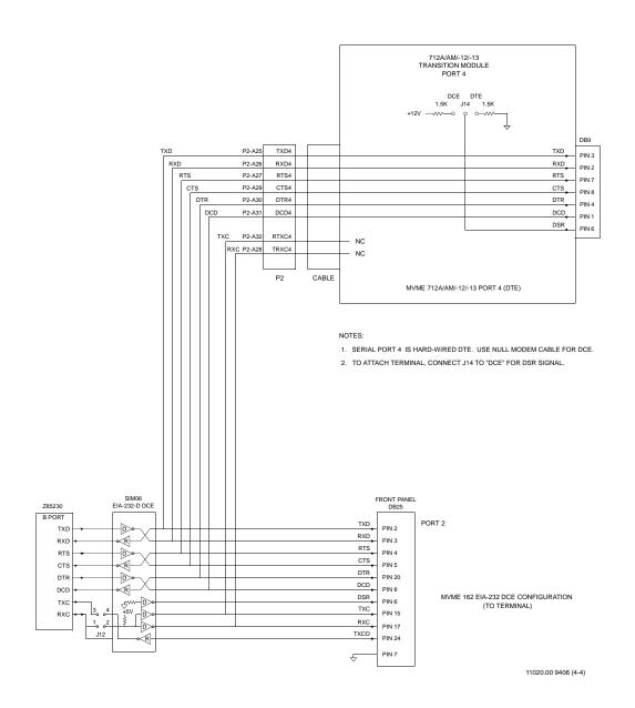
Figure 2-5. MVME162FX EIA-232-D Connections, MVME712A/AM/-12/-13 (Sheet 4 of 4)
