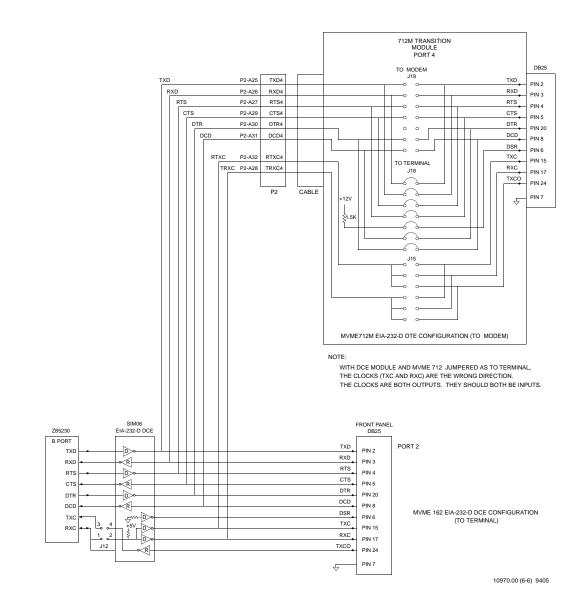
Figure 2-3. MVME162FX EIA-232-D Connections, MVME712M (Sheet 6 of 6)
