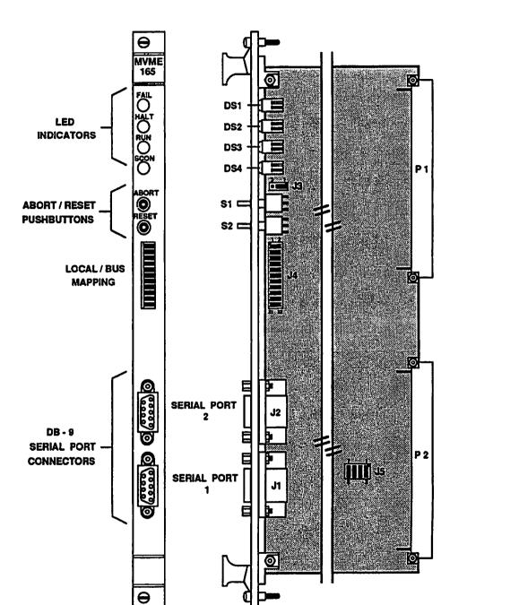
Figure 3-1. MVME165 Front Panel
