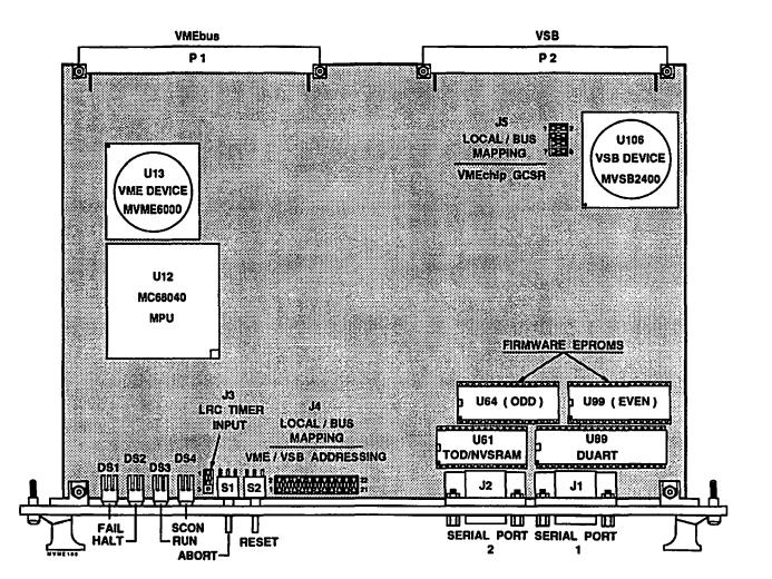
Figure 2-1. MVME165 Jumper, Switch, and Connector Location Diagram
