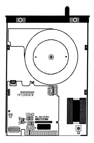
For software selection of speed/density, two jumper changes must be made on the MVME320B: the removal of the jumper on J18 and the installation of a jumper on pins 4-5 of J17 (refer to sections 2.3.11, 2.3.12, and 2.4.c).
