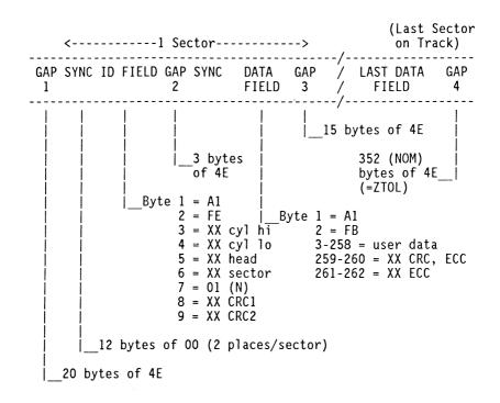
FIGURE A-1. Recommended Hard Disk Track Format (256 Bytes/Sector)
