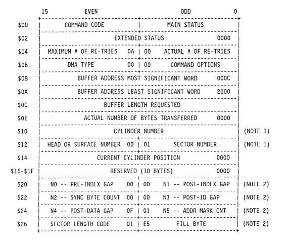
FIGURE B-5. Sample ECA Block Format -- ST412 5-1/4 Inch Hard Disk (10 MHz, 15Mb) B
