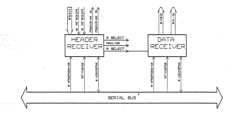
FIGURE 6-7. DATA RECEIVER with HEADER RECEIVER
