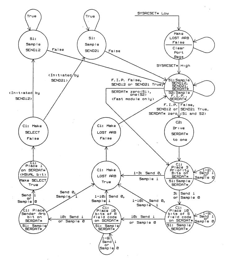
Figure 6-2. HEADER SENDER State Diagram
