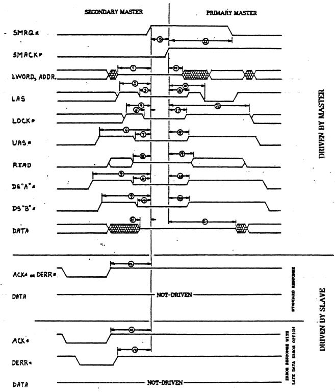
FIGURE 5-5 PRIMARY MASTER receives VMX-DTB: MASTER timing diagram
