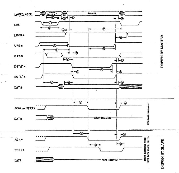
FIGURE 4-1 Single Write Cycle: MASTER timing diagram
