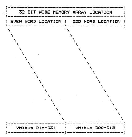
When 32 bits of data are written they are stored in a single longword location. When reading this data 16 bits at a time the even word address (A01 = 0) corresponds to the longword location bits D16-D31.
