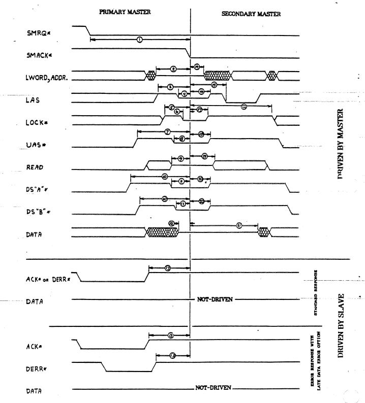
FIGURE 5-3 PRIMARY MASTER grants VMX-DTB: MASTER timing diagram
