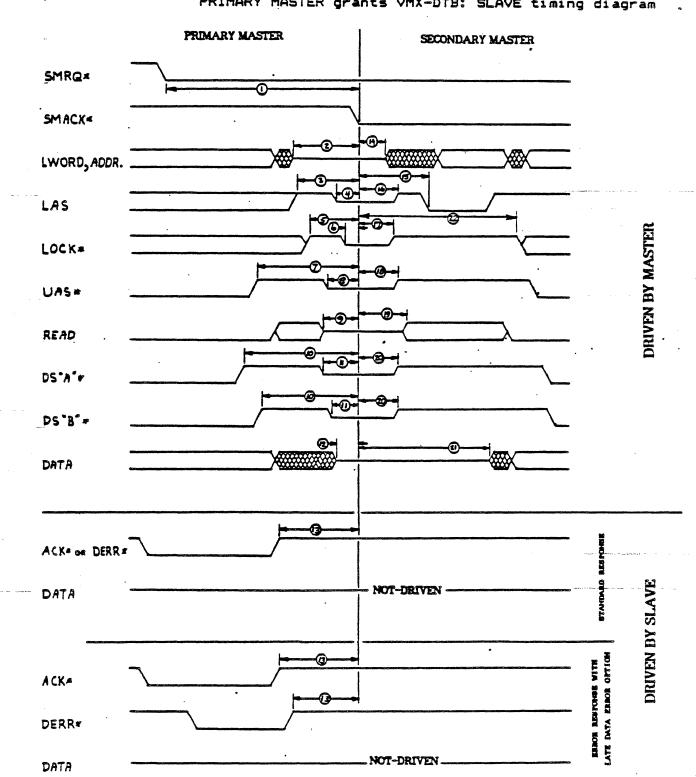
FIGURE 5-4 PRIMARY MASTER grants VMX-DTB: SLAVE timing diagram
