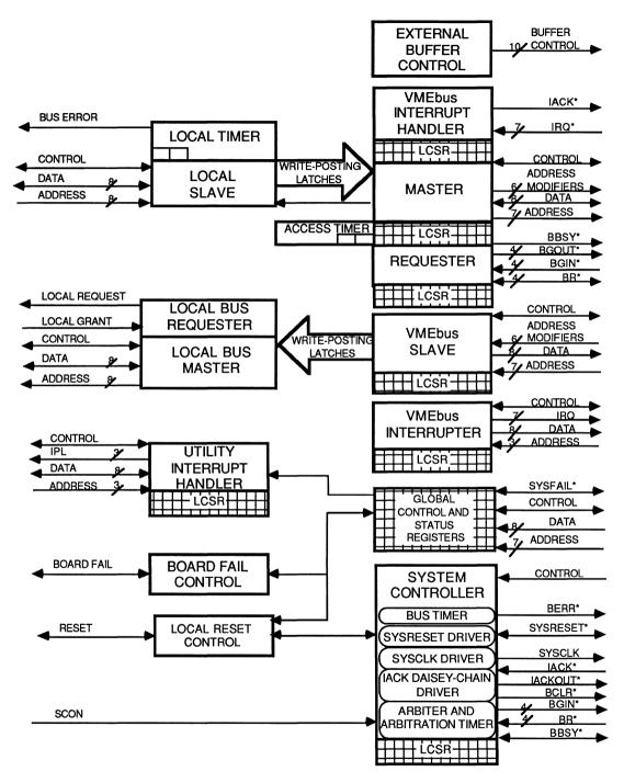
Figure 2-1. Block Diagram of the MVME6000
