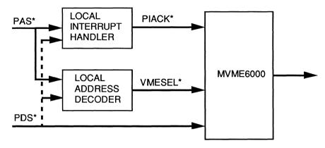
Figure 3-2. Connecting PDS\*, VMESEL\*, and PIACK\* to the MVME6000
