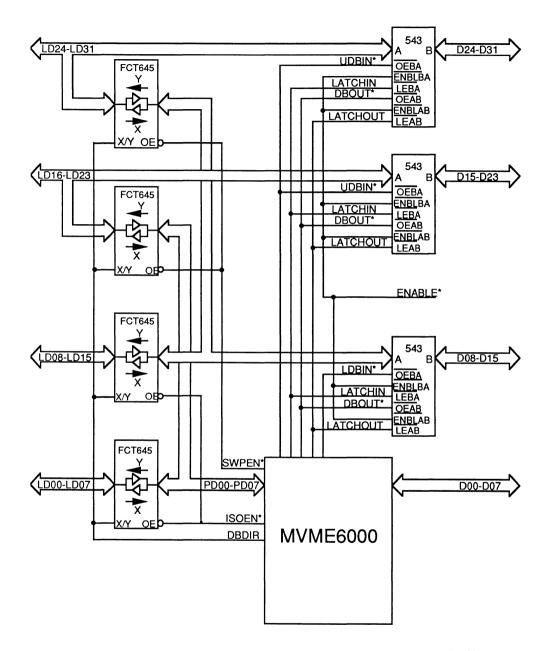
Figure 3-5. Connecting the MVME6000 to External Data Buffers
