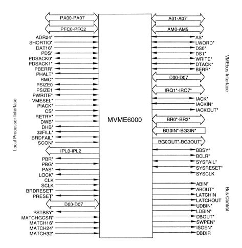
Figure 3-1. Signals of the MVME6000
