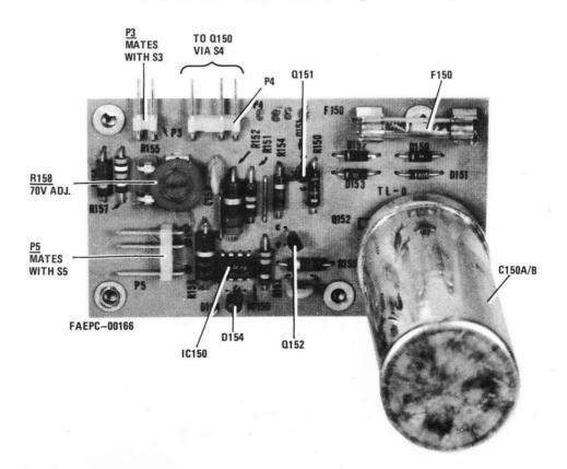
Power Supply Circuit Card (Component View) 4-27
