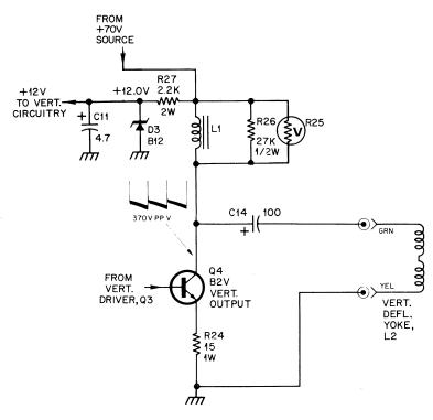
Figure 11. Vertical Output Circuit
