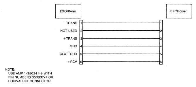
FIGURE 2-1. EXORterm 150/EXORciser Current Loop Interconnection Cable
