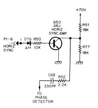
Figure 4. Horizontal Sync Amplifier Circuit
