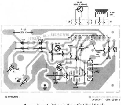
Power Supply Circuit Card (Solder View) 4-28
