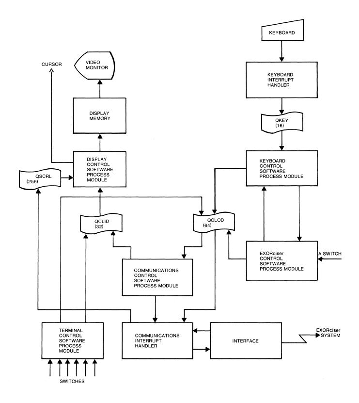
FIGURE 1-4. EXORterm 150 System Flow Chart
