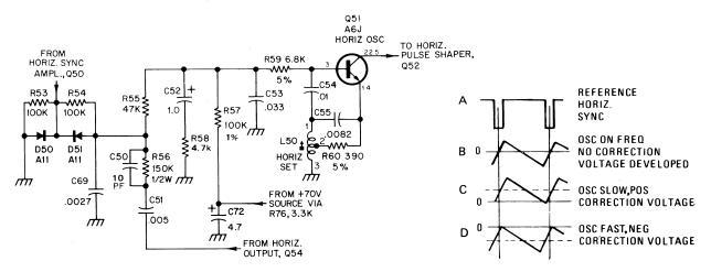
Figure 5. Phase Detector and Horizontal Oscillator Circuits
