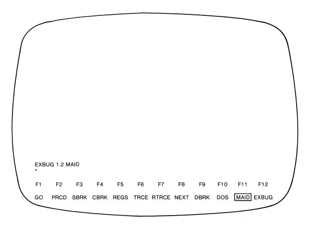
FIGURE 3-4. CRT Display for MAID Command Level Selection
