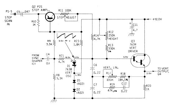
Figure 10. Vertical Oscillator/Driver and StepScan Amplifier Circuits
