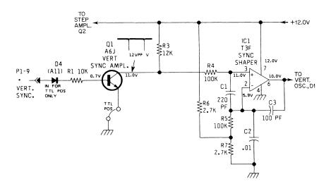
Figure 9. Vertical Sync Amplifier and Sync Shaper Circuits
