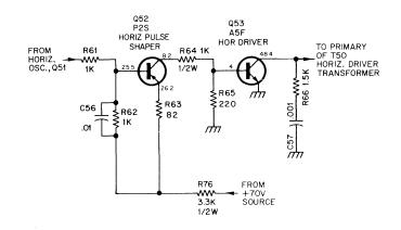
Figure 6. Horizontal Pulse Shaper and Driver Circuits
