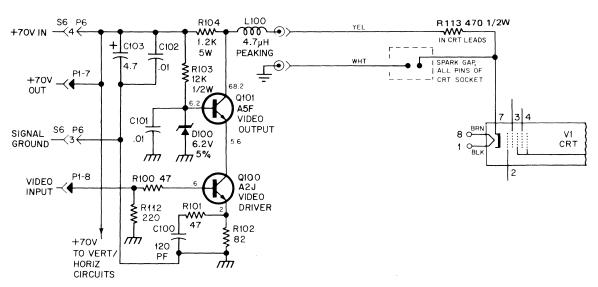
Figure 3. Video Amplifier Circuit
