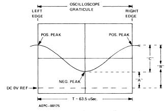
Figure 1. Adjusting Dynamic Focus with an Oscilloscope
