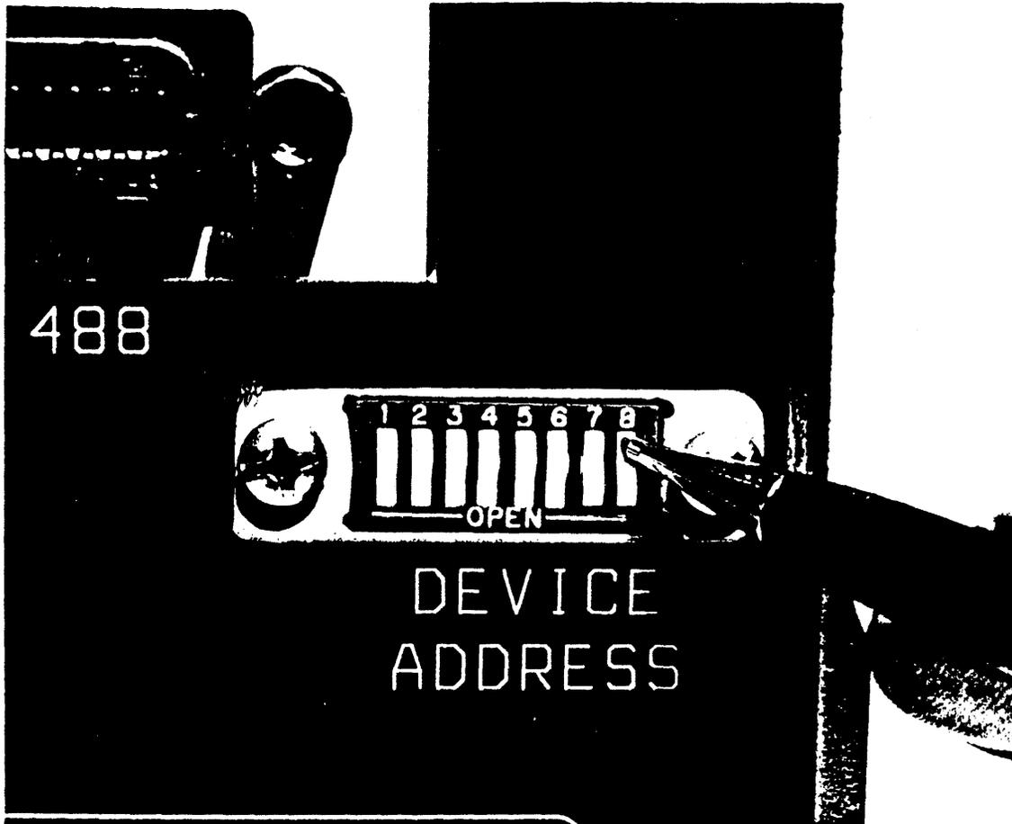
FIGURE 2-5 SETTING DEVICE ADDRESS SWITCHES
