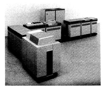
An NCR Century 200 system, with printer in foreground and dual-spindle disc unit at right.
