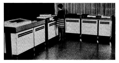
This Century 101 Basic System consists of a 16K central processor, 450-lpm printer, 300-cpm card reader, and dual-spindle disc unit capable of storing up to 8.4 million bytes. Newest of the five Century Series processors, the Century 101 offers more than twice the internal performance of the Century 100 at less than a 50% increase in cost.
