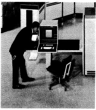
The Century 300's Operator Communication Center, an integral part of the central processor, includes a CRT display, keyboard, printer, and control panel.
