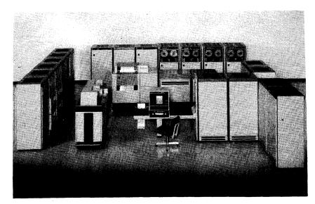
With about twice the internal performance of the Century 200, the Century 251 neatly plugs the sizeable performance gap that previously existed between the 200 and the topof-the-line Century 300. Shown here is a large Century 251 installation with both disc and magnetic tape capabilities.
