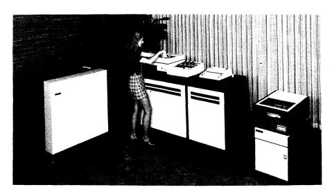
One of the two May 1974 additions to the NCR Century Series computer family, the compact Century 151 is the first to utilize MOS main memory. The Basic System pictured here features 32K bytes of 750-nanosecond MOS memory, an integrated 300-lpm line printer and 300-cpm card reader, and 9.8 million bytes of disc storage.
