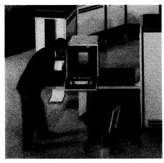
The Century 300's Operator Communication Center, an integral part of the central processor, includes a CRT display, keyboard, printer, and control panel.
