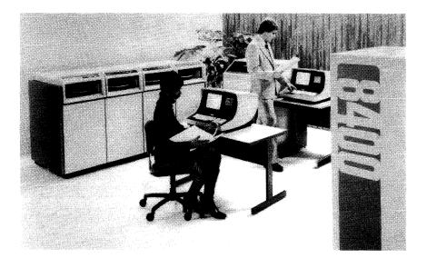
An additional miniprocessor that serves as an intelligent disk interface, plus multiple microprocessors for low-cost communications interfacing.
