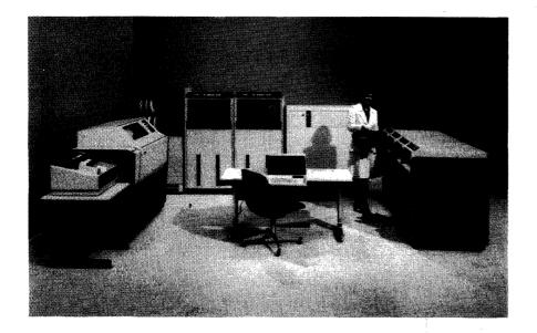
The NCR 8570 was one of the first two 8000 Series systems introduced in April 1976. Originally offered as an NCR Century emulator, this system is now also available in a virtualmemory model designated the V-8570. The configuration shown here includes four 70-megabyte Model 6590 Disk Drives that feature "Winchester-style" data modules similar to IBM's 3348 data modules.
