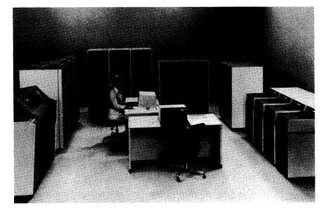
NCR's new V-8500 Group II Series includes seven models that can have from one to four CPUs, one to eight megabytes of memory, and a wide range of I/O devices. Performance is comparable to the IBM 4300 Series.
