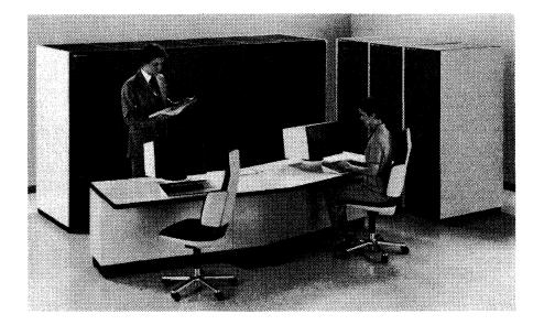
At the top of NCR's product line is the dual-processor V-8670, with 4 megabytes of memory, expandable to 16 megabytes. Processing speed is in the range of five MIPS (million instructions per second), making the V-8670 comparable to the IBM 3033. All NCR systems are air cooled.
