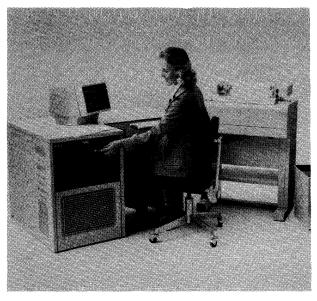
This NCR 8150 configuration consists of a CPU with 48K bytes of MOS memory, 4.9-megabyte cartridge disk drive, visual display terminal with 9-inch screen, keyboard, and serial matrix printer. The 8150 can be expanded to include up to 256K bytes of memory and 39.2 million bytes of disk storage.
