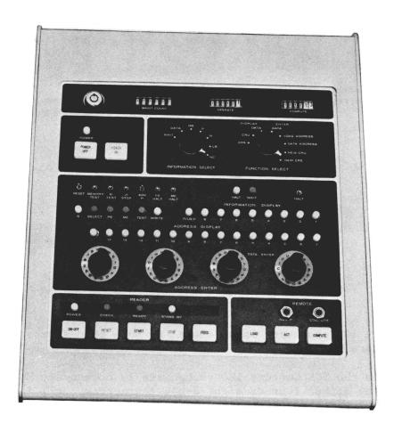
The operator's control panel is the functional control center for the NCR Century 100 System. This panel and its associated components occupy a dedicated position on one of the input/output trunks. The indicators, rotary switches, toggle switches, and push-button switches are logically and conveniently arranged on the panel.
