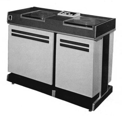
The system dual disc is a magnetic file device with random-access capabilities. It contains two discs, each with its own read/write head assembly on a movable arm. The disc packs may be independently mounted or removed.
