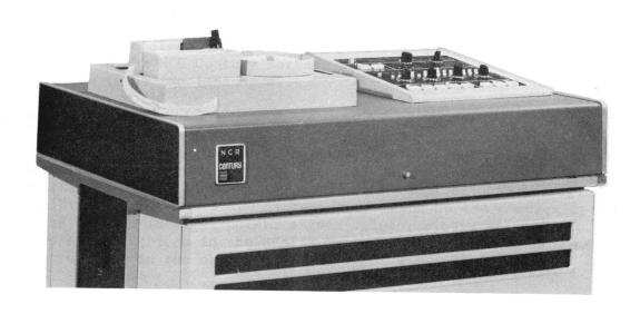
The system paper tape reader, which is basically a strip reader, accepts 5-, 7-, or 8-channel punched paper tape. However, rolls of paper tape up to 300 feet long may also be processed on this paper tape reader. The reading speed is 1000 characters per second.
