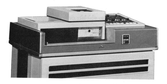
The system card reader reads 300 cards per minute. The feed hopper and output stacker, which have a capacity of 1000 cards each, are easily accessible. The transport mechanism maintains constant contact and control of the cards as it guides them through the reader. This positive card control minimizes card jams and wear.
