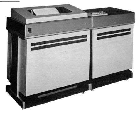
The NCR Century 100 base system has a line printer with a printing speed of up to 450 lines per minute. Each line has 132 columns (print positions). The character-set on the type cylinder of the system printer includes 26 alphabetic characters, 10 numeric characters, 28 special characters, and space.
