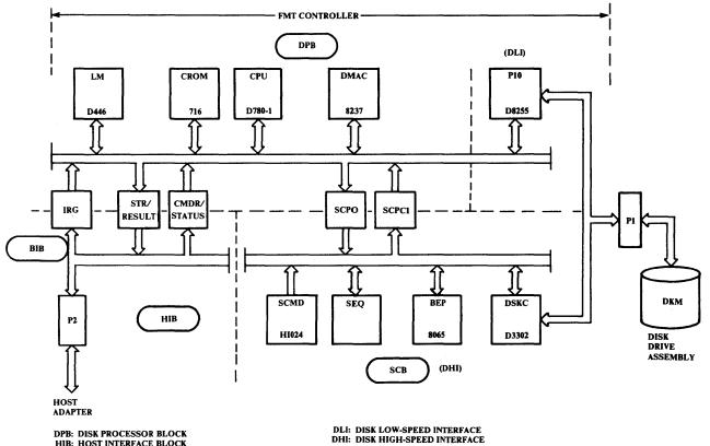
DPB: DISK PROCESSOR BLOCK HIB: HOST INTERFACE BLOCK SCB: SUBCOMMAND BLOCK
