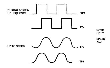
c. With the disk drive at a constant speed adjust RV1 until both waveforms are in phase as shown below. This adjustment sets the spindle motor at its designed speed.
