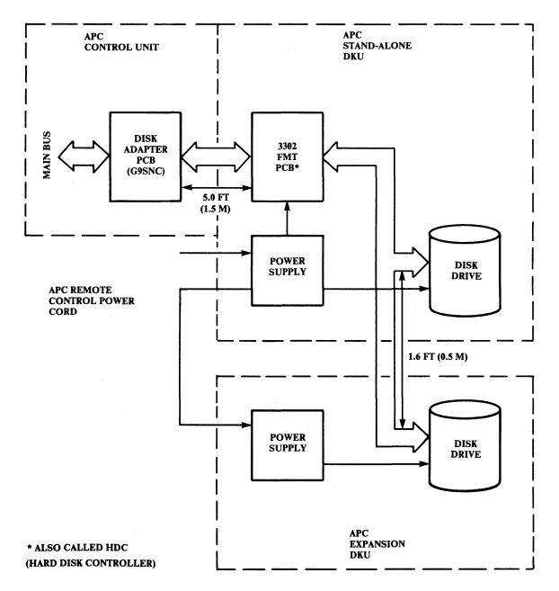
Figure 1-3 APC Stand-Alone/Expansion DKU Functional Block Diagram
