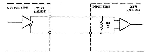
DATA TRANSFER LINE FORMS A DIFFERENTIAL TRANSMITTING AND RECEIVING CIRCUIT.
