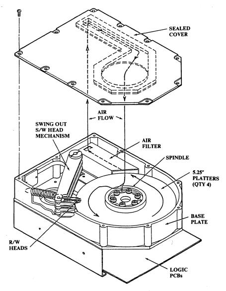
Figure 3-1 APC Disk Module (Exploded View)
