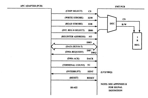
Figure 2-4 Interface Signals (Adapter to FMI)
