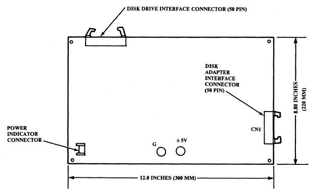
Figure 2-8 FMT PCB Physical Configuration
