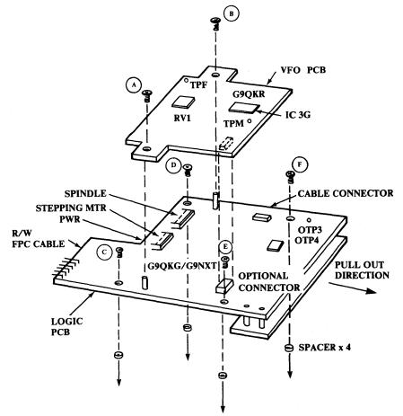
Figure 3-6 PCB Diassembly/Assembly (Disk Drive)
