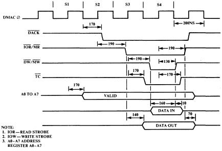
Figure 2-6 DMA Access Timing
