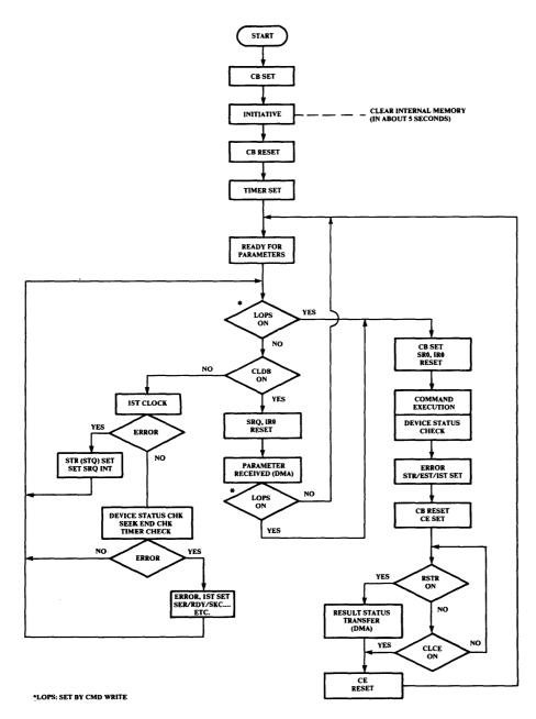
Figure 2-12 FMT Firmware Flowchart
