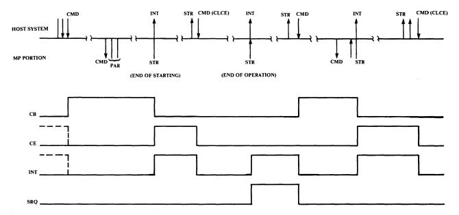
Figure 2-15 Seek/Recalibrate Timing
