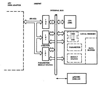
Figure 2-9 Firmware Hardware Interface
