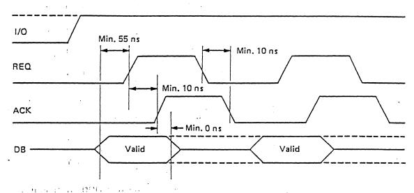
(Fig 3-5.5.2 Data transfer from target to initiator)
