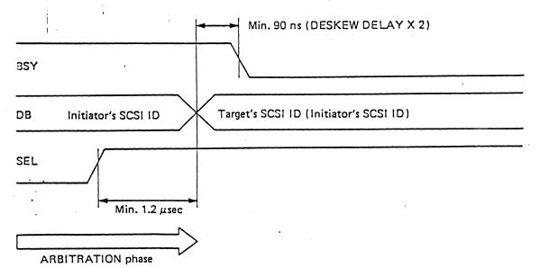
(Fig. 3-3.3.2 Start of SELECTION phase - ARBITRATION phase used)
