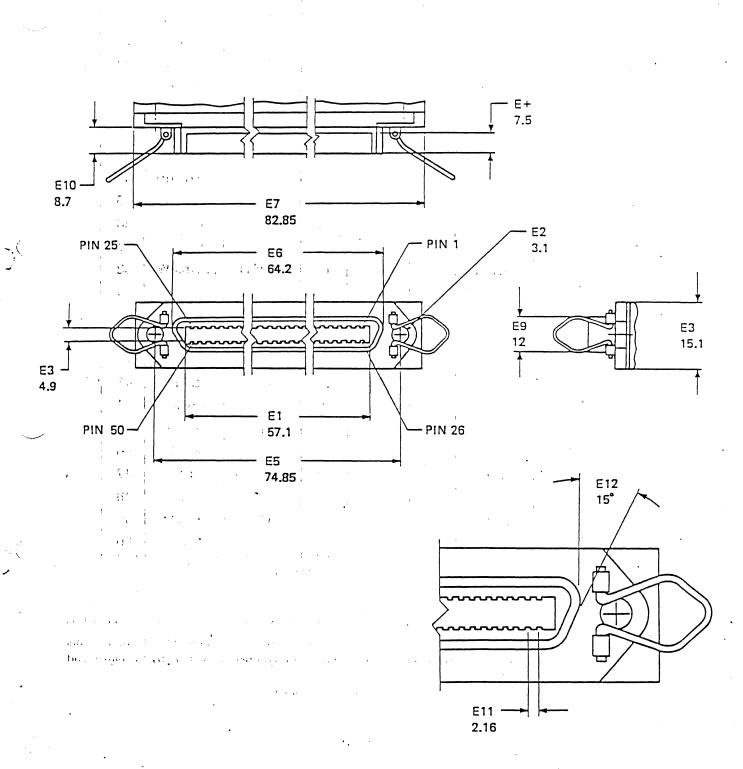
Fig.4-3.1 Shielded SCSI Device Connector (Alternative 2)
