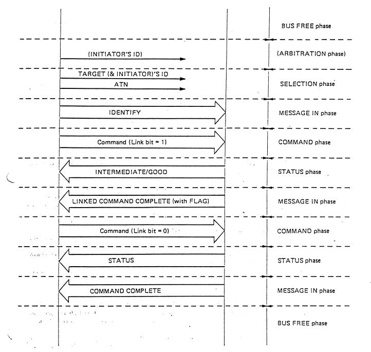
(Fig.6-2.6 Example of command link (two TYPE 1 commands)
