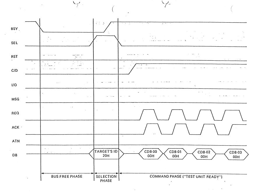
Fig. 6-2.7.1 Example of bus phase operation-1
