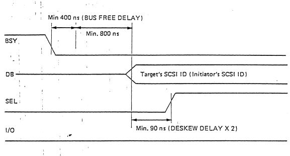
(Fig. 3-3.3.1 Start of SELECTION phase - no ARBITRATION phase used)
