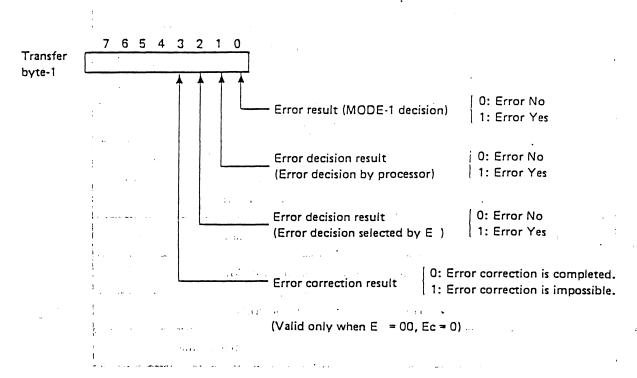
However, this function is only valid for the READ (C8H) command. The EXTEND READ command does not send the sector status.
