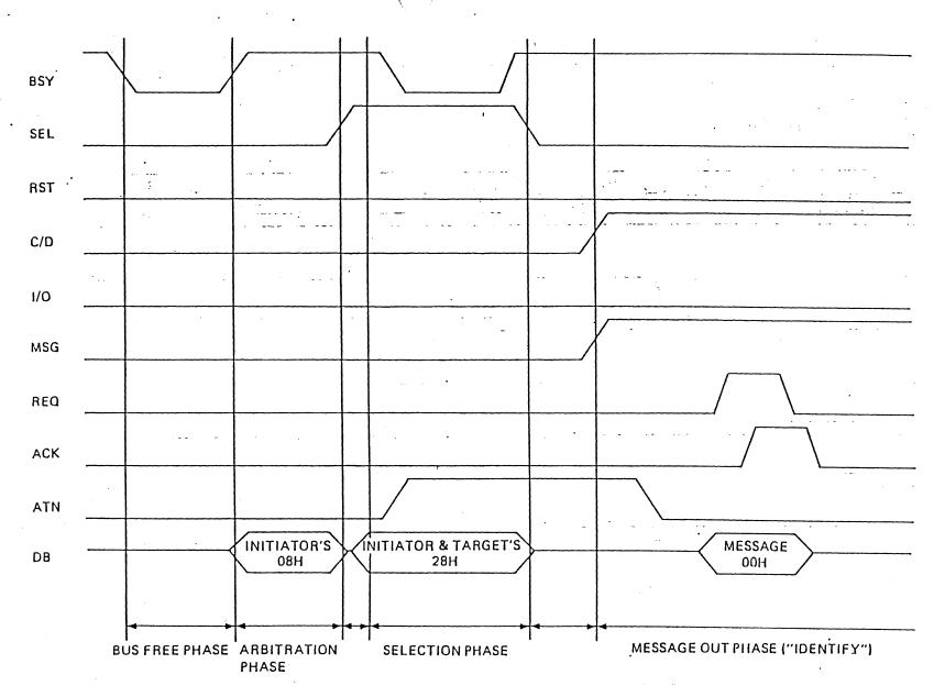
Fig. 6-2. 7.2 Example of bus-phase operation-2
