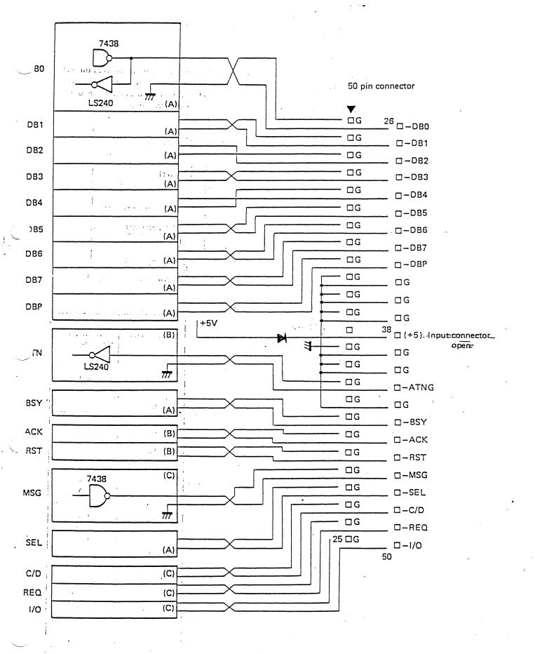
Fig.4-5 Interface drive circuit, recieve circuit, and pin connector arrangement.
