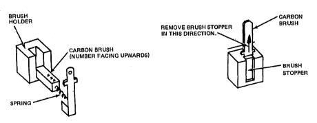
Figure 4-13 Removing a Carbon Brush
