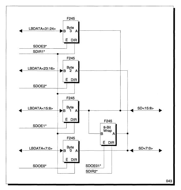
Figure 19 VL-Bus to ISA-Bus Data Transceivers
