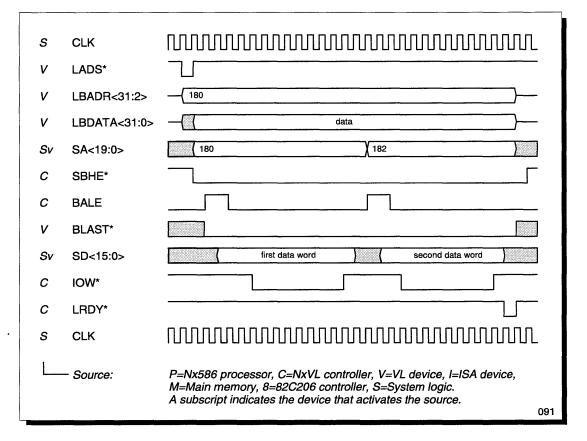
Figure 48 VL-Master 32-Bit Write to ISA-Bus 16-Bit I/O
