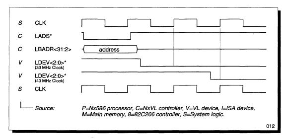
Figure 39 Response by a VL-Bus Device to Address Strobe
