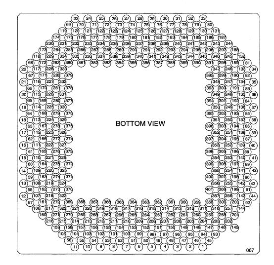
Figure 7 NxVL Pinout Diagram (Bottom View)
