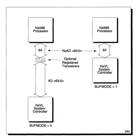
Figure 14 NxVL Connection Alternatives to the NexBus
