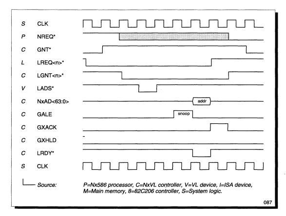
Figure 44 Bus Arbitration by VL-Bus Master
