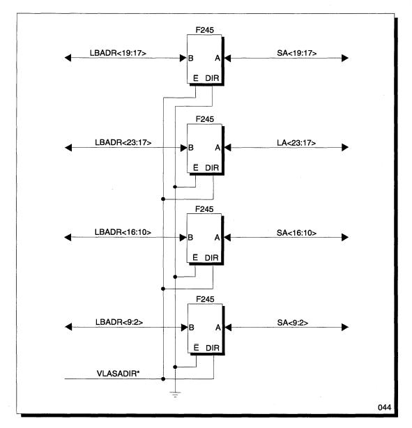
Figure 20 VL-Bus to ISA-Bus Address Transceivers
