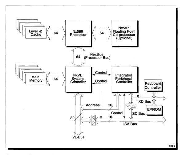
Figure 9 System Block Diagram
