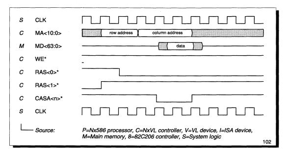
Figure 60 Slow Read from Main Memory (Overlapping Precharge)
