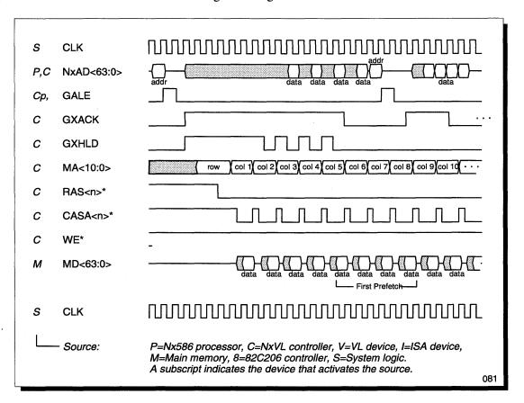
The example assumes that fast DRAM accesses are enabled by setting bits 12 and 22 of the configuration register CFG0 to 1.
