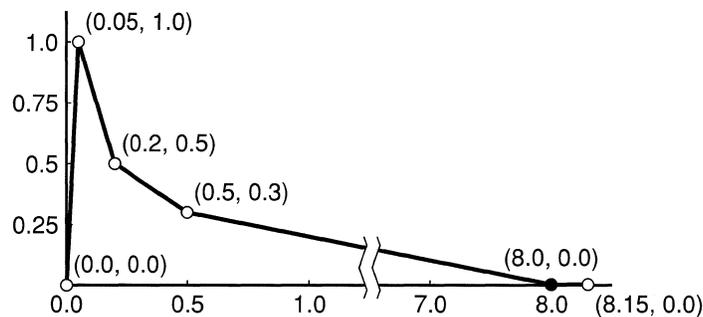
Figure 3-11. Simulated Piano Envelope
