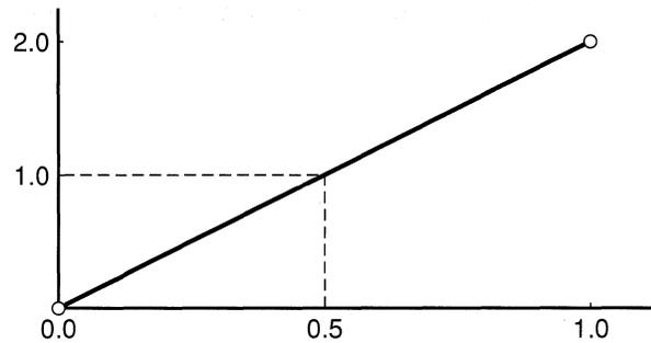
Figure 3-13. Linear Interpolation
