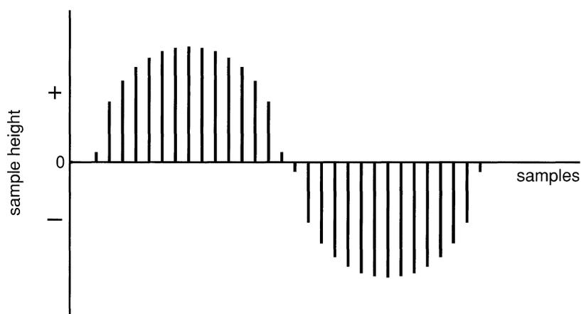
Figure 2-2. Sampled Waveform
