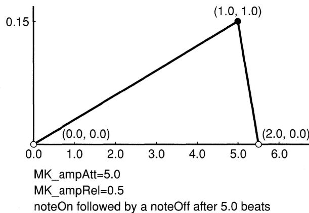
Figure 3-8. Envelope with Attack and Release
