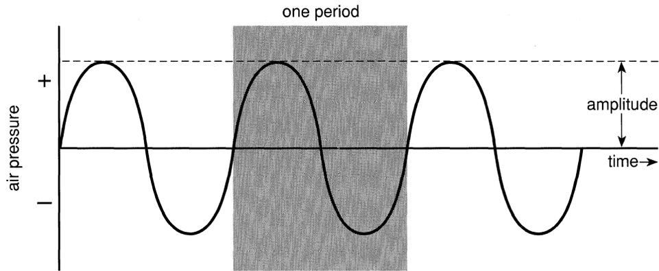
Figure 2-1. Air Pressure Wave
