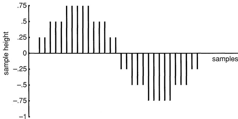
Figure 2-3. Three-Bit Quantization
