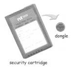
Amber includes the use of a "dongle", essentially an electronically-readable serial number embedded in something that looks like an oversized watch battery, which must match the number the software expects to see. It provides a measure of protection against software piracy. The dongle replaces the older, larger security cartridge, which used to have to be upgraded with each new addition to a switch's functionality.
