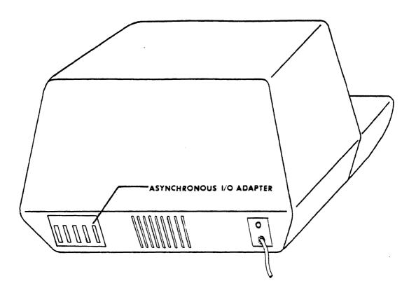
Figure 7R-1. External Connector to Asynchronous I/O Adapter
