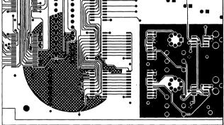
The circular copper pour has a cross-hatch pattern with the hatch grid of 50 at a 45 degree rotation.
