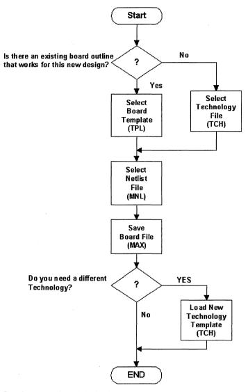
The diagram below illustrates the process for opening a new design.
