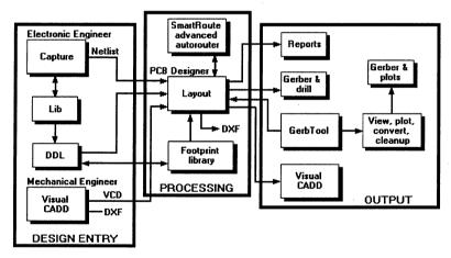
The printed circuit board design flow.
