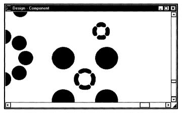
Viewing thermal connections.
