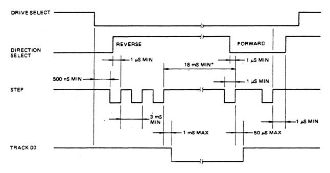
\*NOTE: Turn around time is 18 mS (MIN) when direction is changed.
