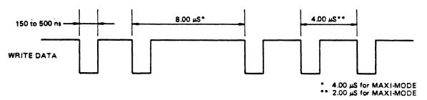
FIGURE 54 WRITE DATA TIMING
