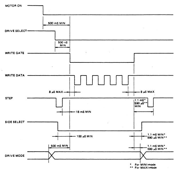
FIGURE 5-3 WRITE INITIATE TIMING
