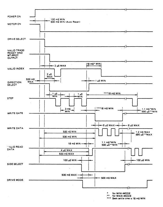
FIGURE 5-6 GENERAL CONTROL AND DATA TIMING
