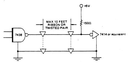
FIGURE 2-2 INTERFACE SIGNAL DRIVE/RECEIVER
