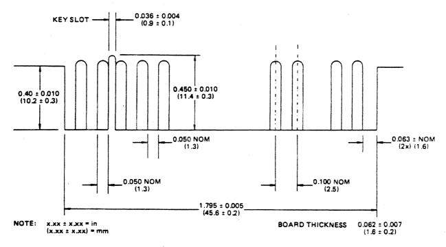
FIGURE 6-2 J1 CONNECTOR DIMENSIONS
