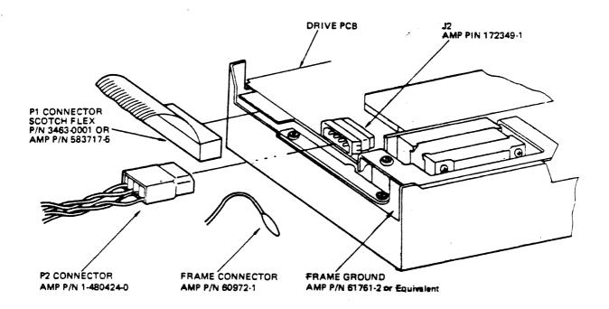
FIGURE 6-1 INTERFACE CONNECTORS LOCATIONS
