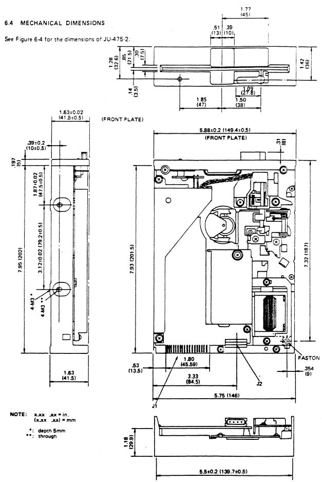
FIGURE 6-4 MECHANICAL DIMENSIONS
