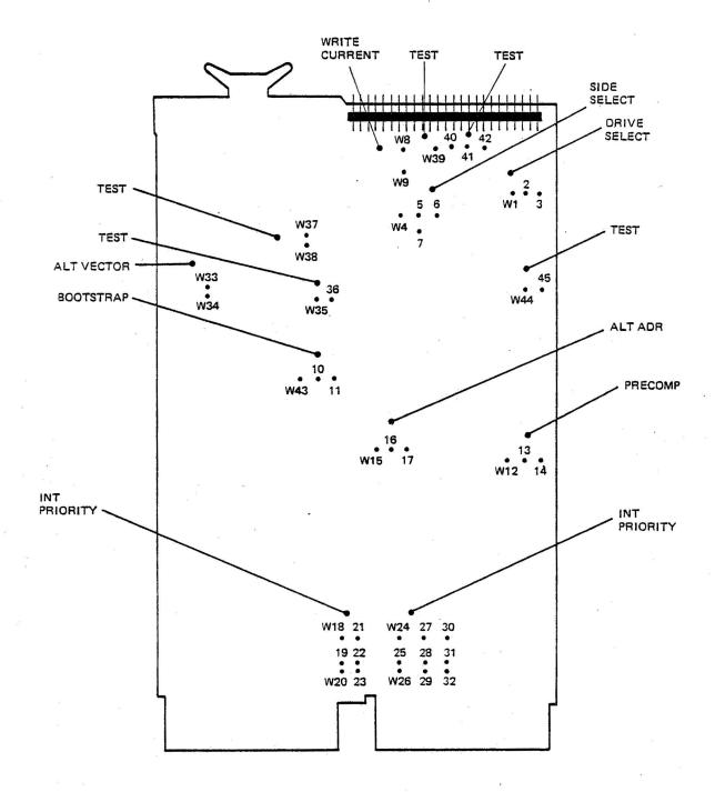
Figure 2-1. PM-XCV21/XCV31 Configuration Jumper Locations
