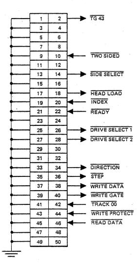
Figure 2-3. Connector Pin Definitions
