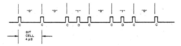
Figure 1-2. FM Recording Characteristics
