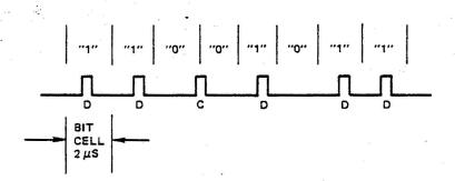
Figure 1-3. MFM Recording Characteristics
