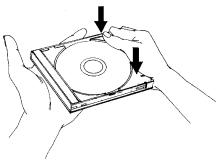
If the caddy appears defective (e.g., warped, cracked, or bent) do not Caution: insert it into the drive. A defective caddy can become stuck inside the drive, requiring the drive's return to your dealer for service. If your caddy appears defective, promptly replace it with a new one.
