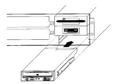
You now need to make the power connection. In most computers you will find additional power connectors that are ready for your use. Check the cable running from your power supply to your hard disk and see if it has extra connectors on it. If so, you can plug one of these into the power connector found on the rear panel of the CD-ROM drive.
