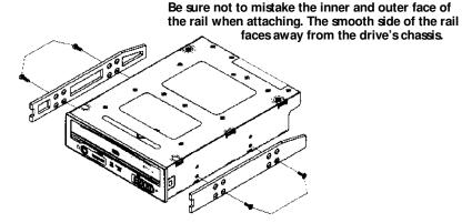
There are 4 holes provided on each side of the drive. To mount an internal drive in most computers, the rails should be fastened to the lower pair of holes. In some instances you may need to fasten the rails to the upper set of holes.
