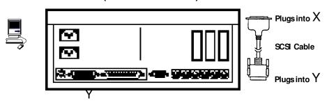
If you are installing more than one PX-65CS external drive (or one PX-65CS and other external SCSI peripherals), connect them as shown below:
