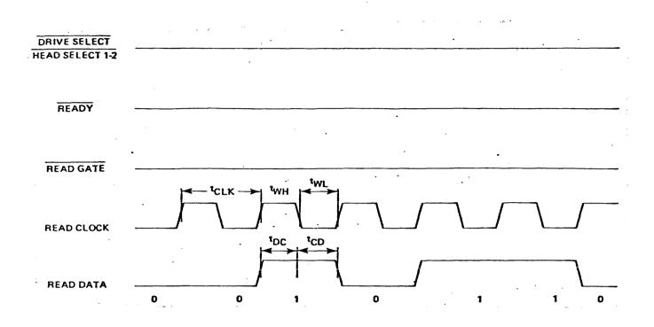
READ DATA and READ CLOCK timing relationship is shown in Figure 12 and their AC characteristics are listed in Table 22.
