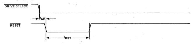
Figure 9. Reset Pulse Width Timing
