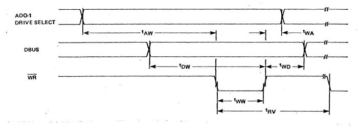
Figure 7. Register Load Timing
