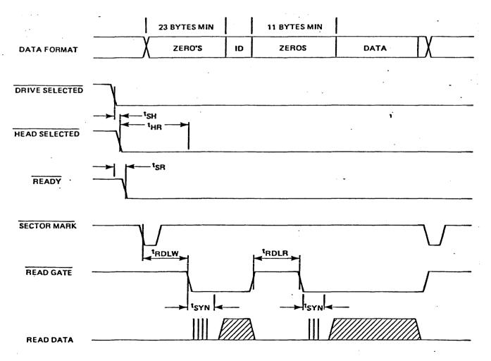
Figure 14. Record Reading Timing
