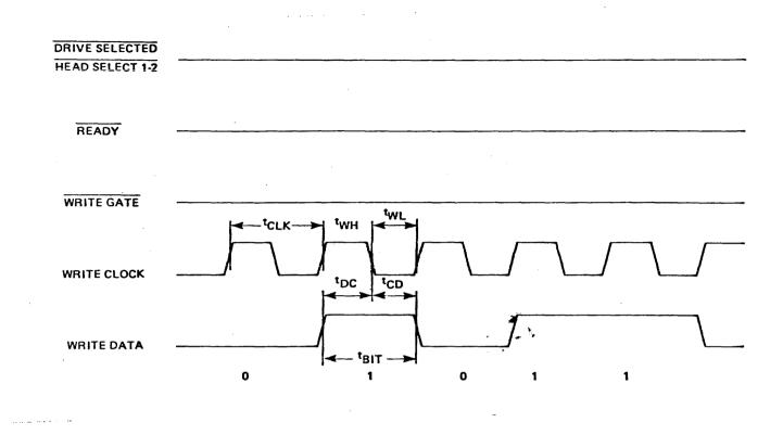
Figure 11. WRITE DATA and WRITE CLOCK Timing
