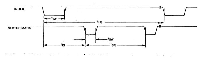
Figure 10. INDEX and SECTOR MARK Timing
