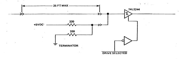
Figure 3. Single Line Receiver Gated By Drive Select
