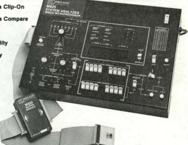
The Analyzer allows examination of the system (address, data, and status) during a user-specified machine cycle at the desired Compare Address. Observation of the system is possible at full system speed or by single-step by instruction or machine cycle. The possible display modes are: dynamic mode, in which the processor continues to run without analyzer interference, and static mode, in which the analyzer controls the processor WAIT line.
