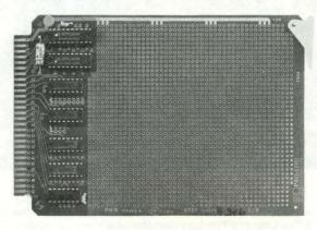
7904 Decoded Input/Output Utility Card
