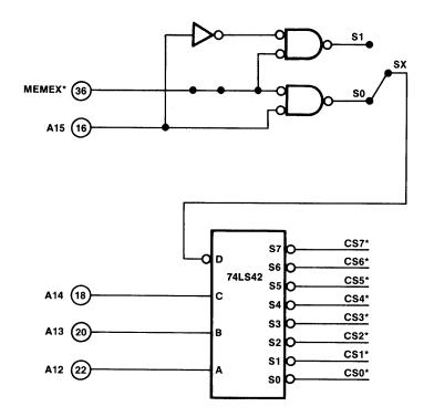
Figure 2-13A Address Decoder Schematic For 4K Memory Blocks (32K Memory Card)
