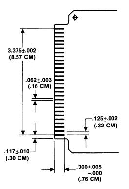
Figure 2-1B Series 7000 STD BUS Edge Card Finger Specifications
