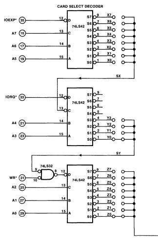
Figure 2-15A I/O Address Decoder And Schematic For 1 Address Per Card
