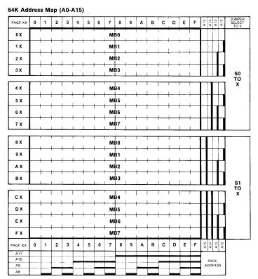
Figure 2-13B Memory Address Map & Jumper Selection Table For 4K Memory Block (32K Memory Cards)
