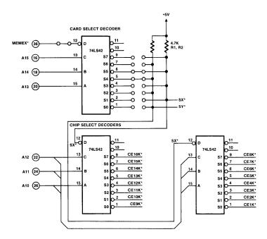
Figure 2-11A Address Decoder & Schematic For 1K Memory Blocks (16K Memory Card)
