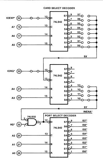
Figure 2-18A I/O Address Decoder And Schematic For 8 Addresses Per Card
