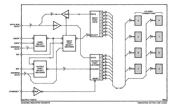
The 7604 is shipped fully populated. The card is customized (to A input and B output ports such that A + B = 8 ports) by removing the unused input buffer or output port latch according to the following table.
