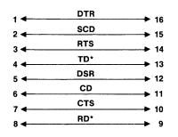
Data Terminal/Data Set Select Plug P1 Wiring Shorting Bars Exposed For Scope Test Points
