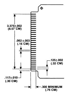
Figure 1-7B Recommended Edge Card Finger Design
