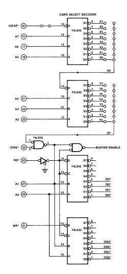
Figure 2-17A I/O Address Decoder And Schematic For 4 Addresses Per Card
