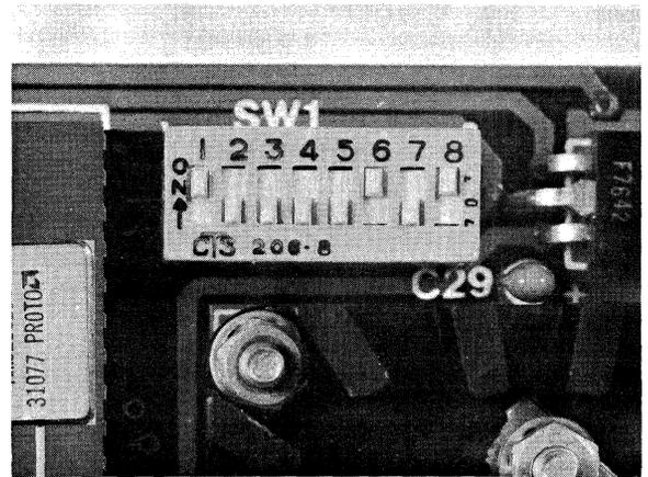
Figure 9. GPM Switches
