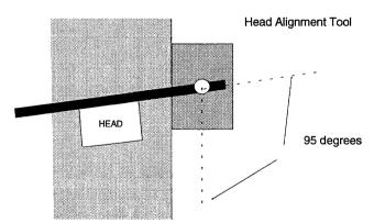
Figure 7-6 Head Alignment Angle
