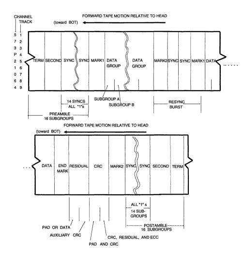
Figure 2-3 GCR Data Tape Format
