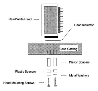
Figure 6-8 Head Mounting Hardware
