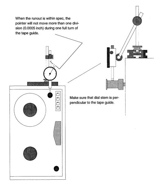
Figure 8-5Measuring Tachometer Tape Guide Runout
