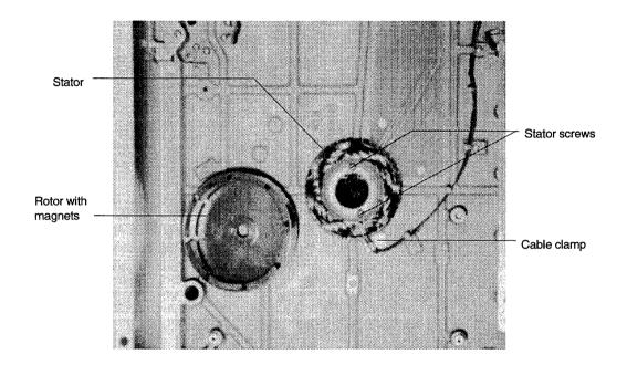
Figure 6-5 Motor Rotor and Stator
