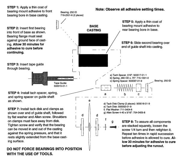
Figure 8-2 Tachometer Tape Guide Assembly
