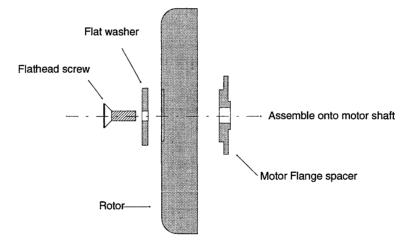
Figure 6-6 Rotor Assembly
