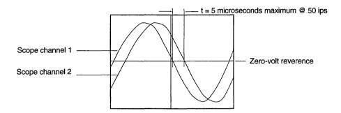
Figure 7-7 Skew Adjustment Waveform
