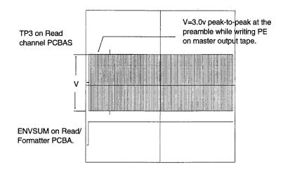
Figure 7-5 Read and ENVSUM Waveforms
