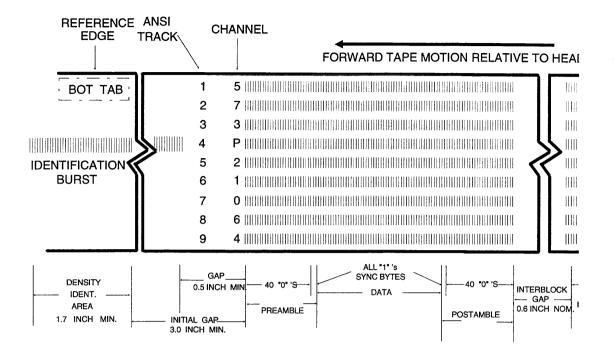
Figure 2-1 PE Data Tape Format
