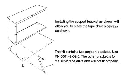
Figure 8-6 Support Bracket Installation
