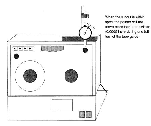
Figure 8-7 Measuring Fixed Tape Guide Runout
