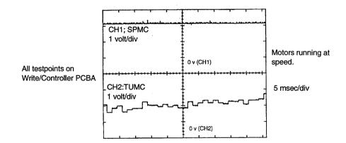
Figure 3-5 Supply and Take Up Motor Waveforms
