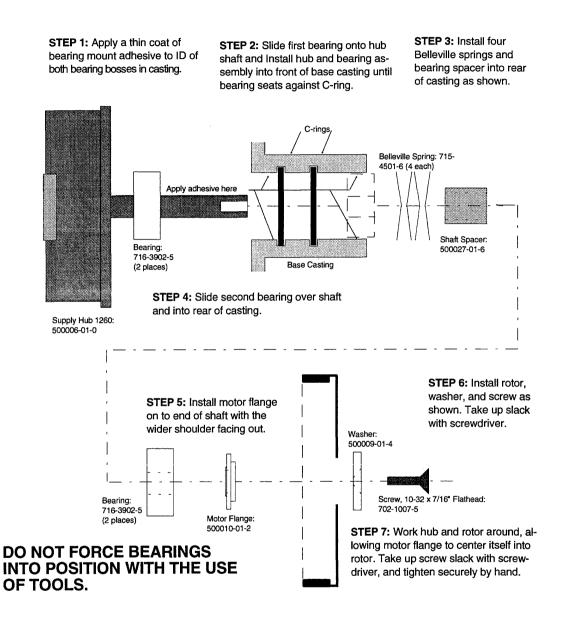
Figure 8-1 Motor Bearing and Component Assembly
