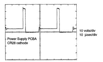
Figure 3-12 +5 Volt Regulator without Load
