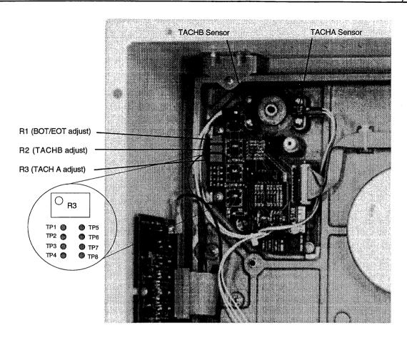
Figure 7-1 Switch PCBA and Tachometer Sensor Locations
