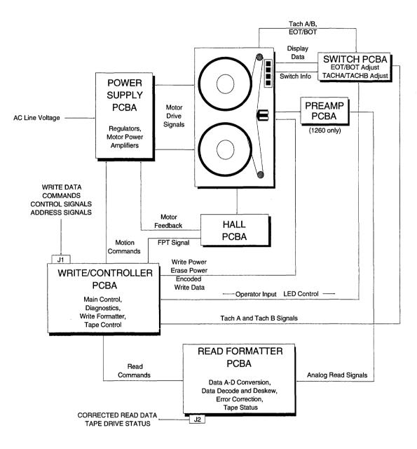
Figure 3-2 1260 Functional Block Diagram
