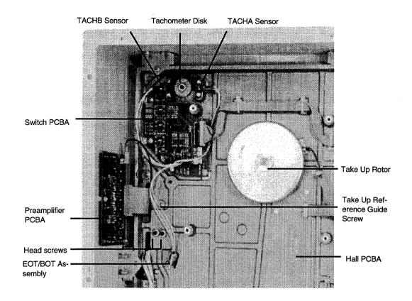
Figure 6-4 Open Drive with Mechanical Parts Identified
