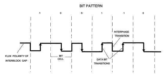
A "1" bit transition is in the direction of the erased tape polarity. A "0" bit transition is in the opposite direction.
