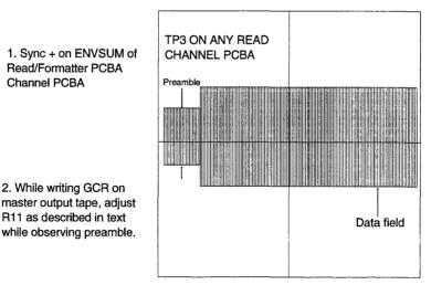
Figure 7-4 GCR Write Current Adjustment Waveform
