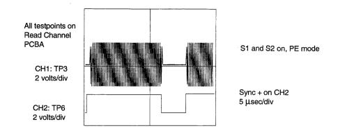
Figure 3-4 Read Analog and Envelope Waveforms
