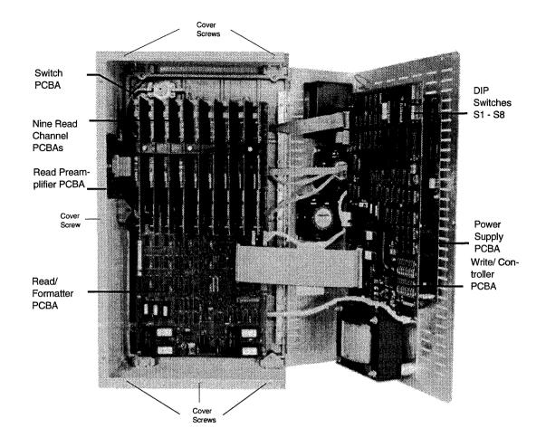
Figure 6-1 Printed Circuit Board Identification
