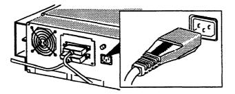
Figure 3-2 Power Connector Location
