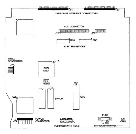
Figure 8-7 SCSI Single-Ended PCBA Layout – 500561 PCBA
