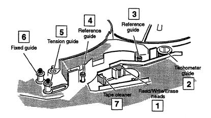
Figure 5-1 Tape Path Components Which Must Be Cleaned
