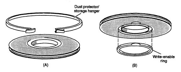
Figure 3-3 Dust Protector and Write Enable Ring
