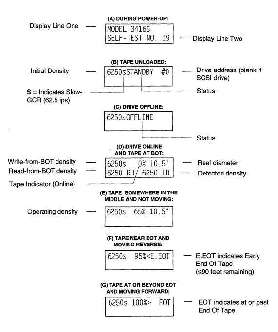
Figure 2-2 LCD during Various Phases of Operation
