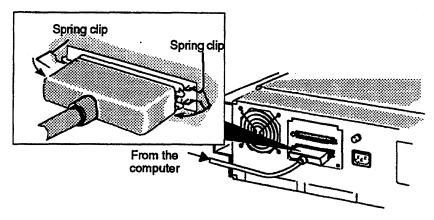
Figure 8-2 Connecting the SCSI Cable to the Tape Drive (SCSI Alternative 2 shown)
