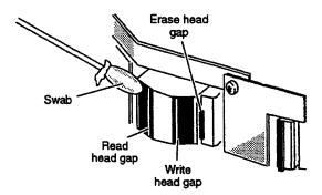
Figure 5-2 Cleaning the Read/Write Head
