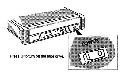
Figure 3-1 Power Switch Location
