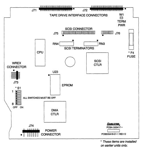
Figure 8-6 SCSI Single-Ended PCBA Layout – 500417 PCBA
