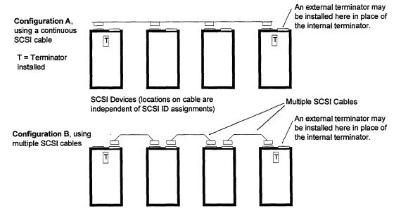
Figure 8-1 SCSI Cable Configurations
