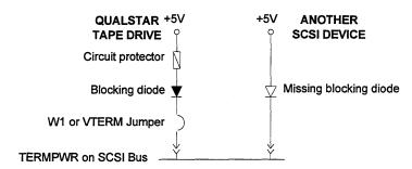
Figure 8-4 Diagram of SCSI Termination Power
