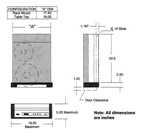
Figure 1-6 Mounting Dimensions
