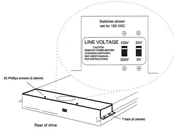
To remove, slide rear cover to rear and lift.
