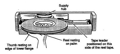
Figure 3-5 Correct Way to Insert Reel
