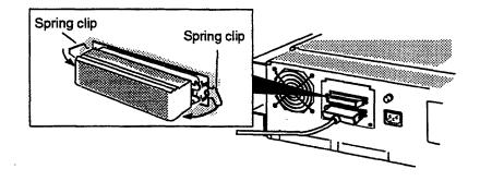
Figure 8-3 Installing an External Terminator
