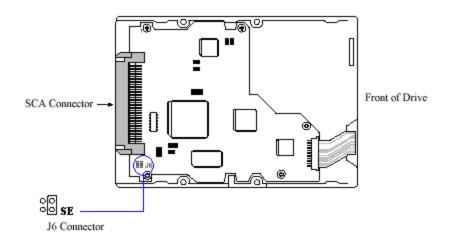
The Viking II SCA drive has only the single jumper position referenced above. Jumper position J6 determines if the drive is forced into SE mode only (jumper in) or if the drive supports multi-mode LVD (jumper out).
