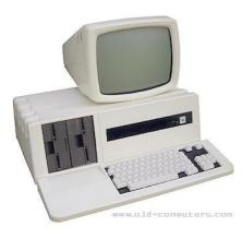
It's a PC based on Zilog Z80A, with 64k RAM, two 256Kb or 600 Kb 5"1/4 floppy disks, 14" monitor monochrome 80x24 text resolution.
