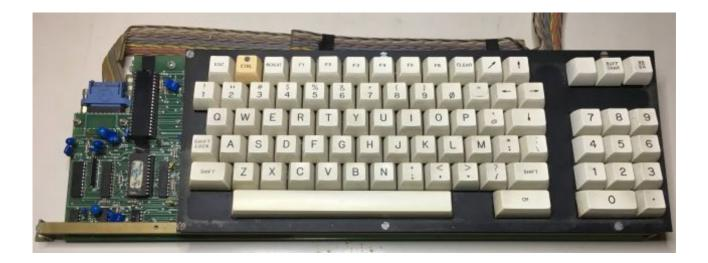
The keyboard communicates with the mother board with a flat cable, probably with a parallel interface; but the peculiarity, which is shown only by removing the tape on the main chip, is that it is driven by another Z80, manufactured by NEC.
