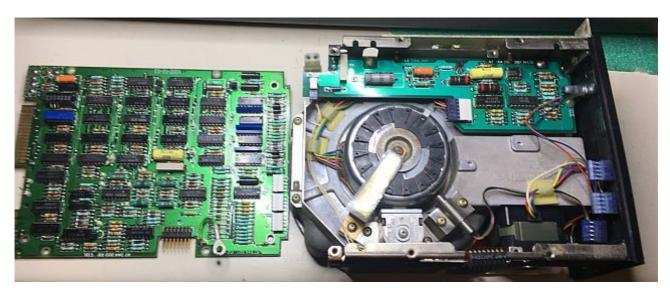
While I was trying to rotate the main motor with my hands, I realized immediately that it was hard to move. I tried to power on the motor and I had the confirmation that was impossible to spin.
