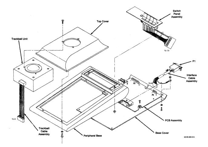
Figure 2-2. Trackball Controller, Exploded View
