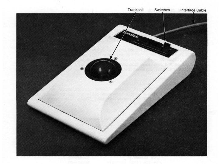
Figure 2-1. Trackball Controller
