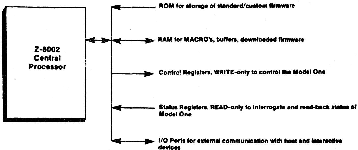
Figure 4.1 Central Processor Addressing and I/O
