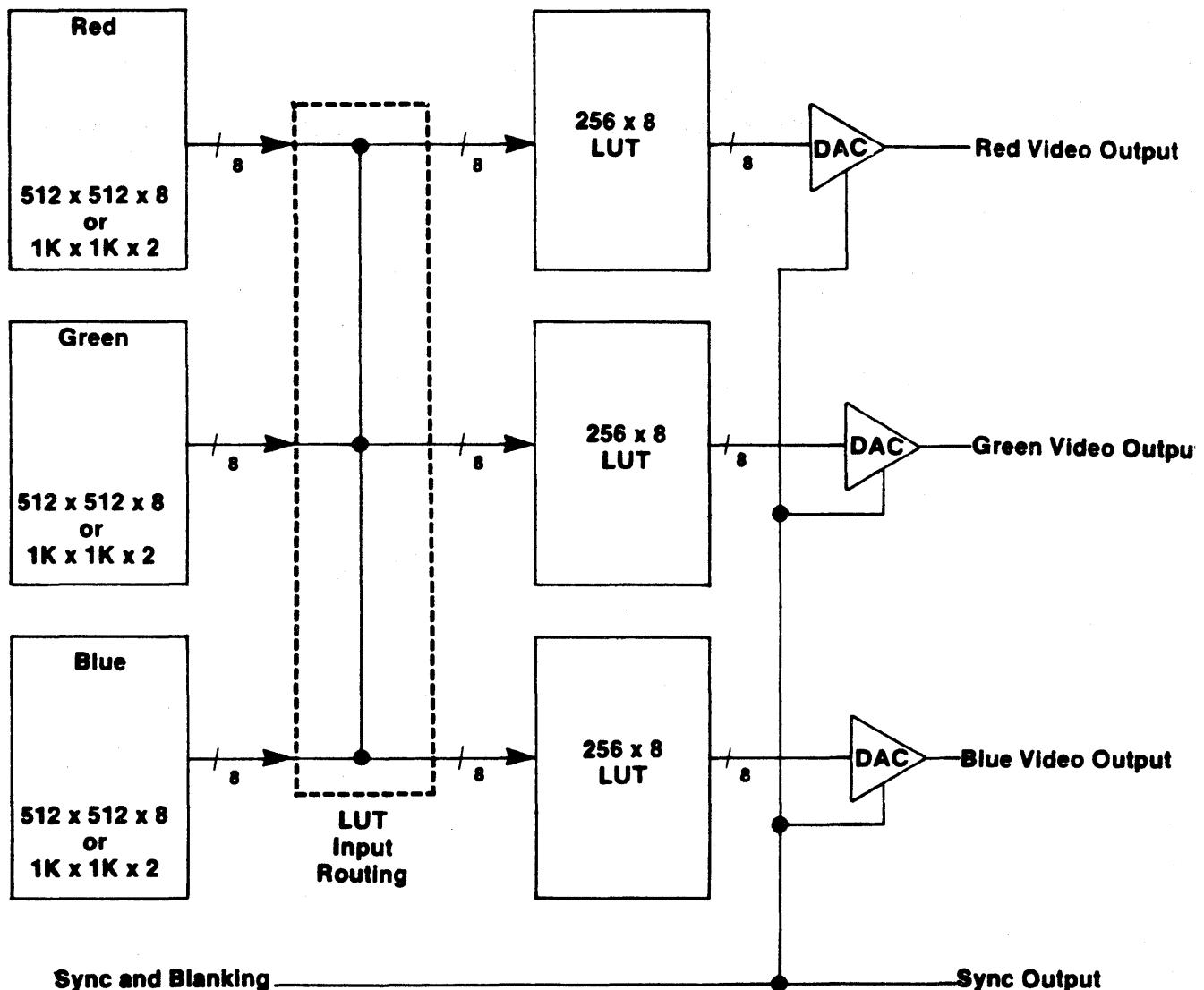
Figure 8.1 Image Memory Output Diagram for the Model One/25
