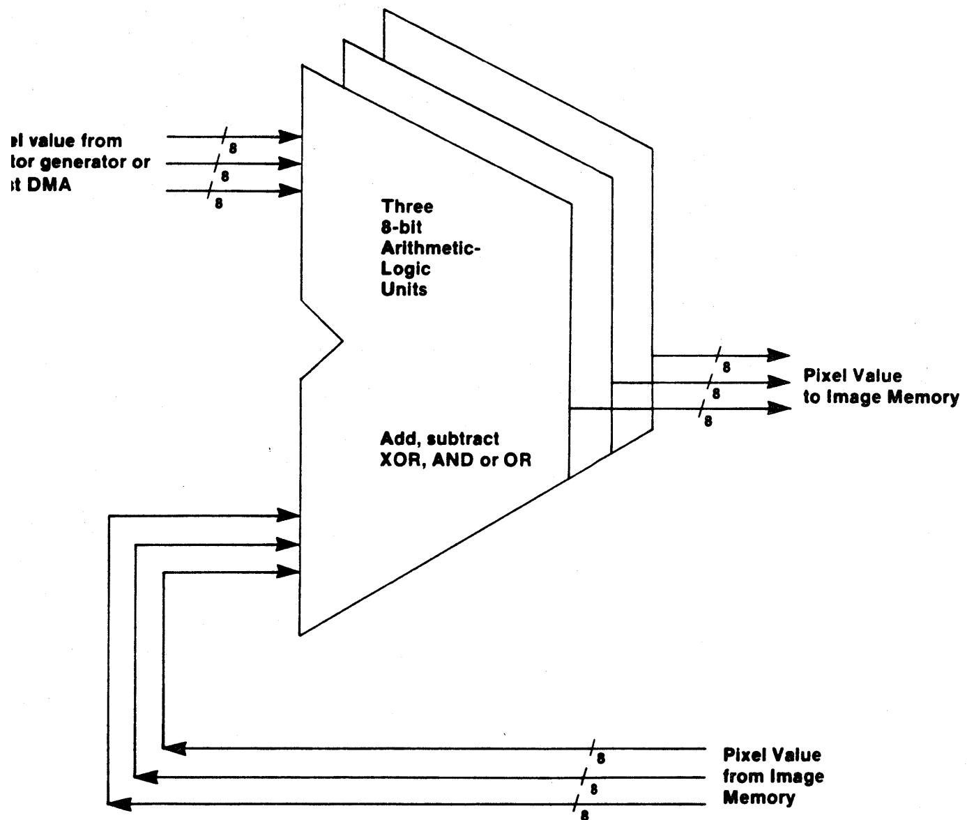
Figure 6.1 Pixel Processor Data Paths
