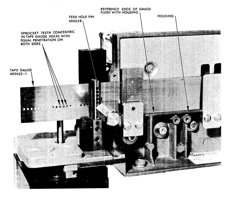
Figure 5-3. Sprocket Alignment Using Tape Gauge.
