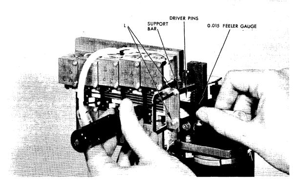
Figure 6-5. Adjustment of Support Bar and Support Bracket.
