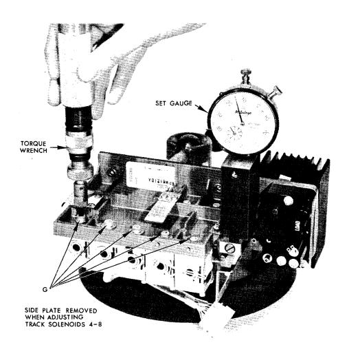
Figure 5-6. Setting Punch Pin Depth.
