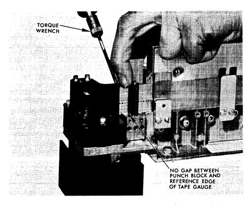
Figure 6-4. Installation of Punch and Pin Block Assembly.
