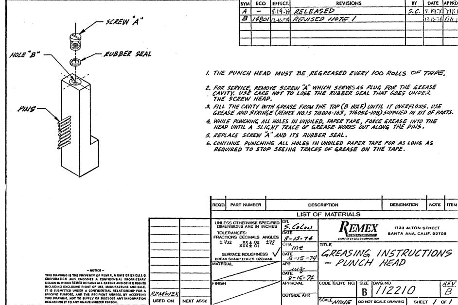
Figure 5-1. Punch Head Greasing Instructions.
