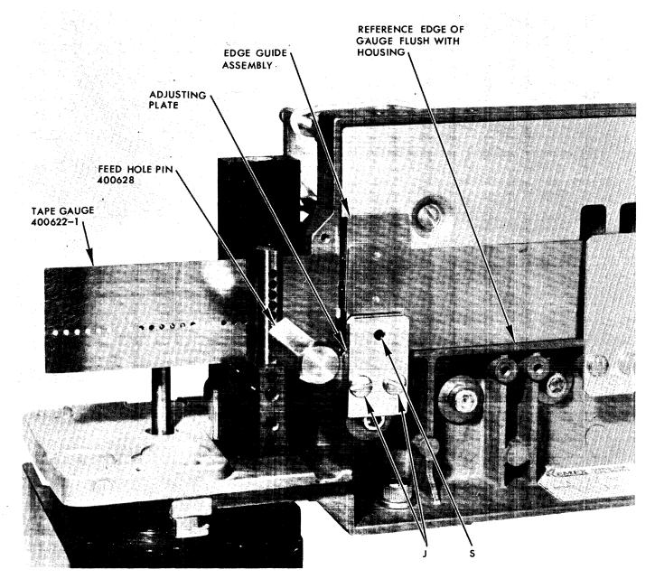
Figure 6-1. Tape Guide and Edge Guide Assembly Alignment.
