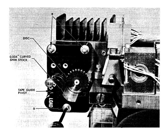
Figure 5-4. Tape Drive Assembly Alignment.
