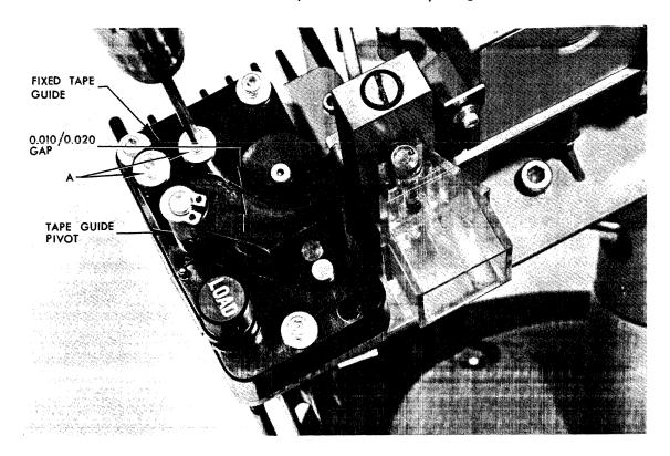
Figure 5-5. Fixed Tape Guide Alignment.
