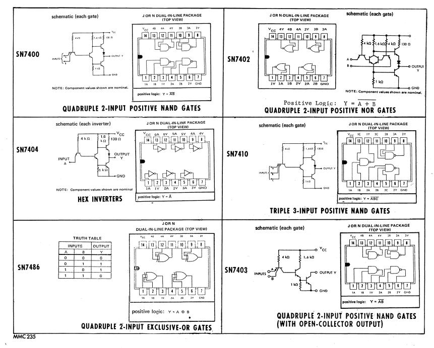
Figure 8-12. IC Assembly Modules Used on the Circuit Cards
