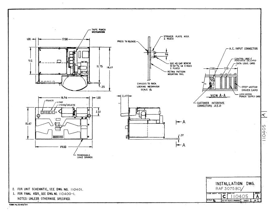
Figure 1-4. Installation Drawing, Model RAF3075 and RDF3075
