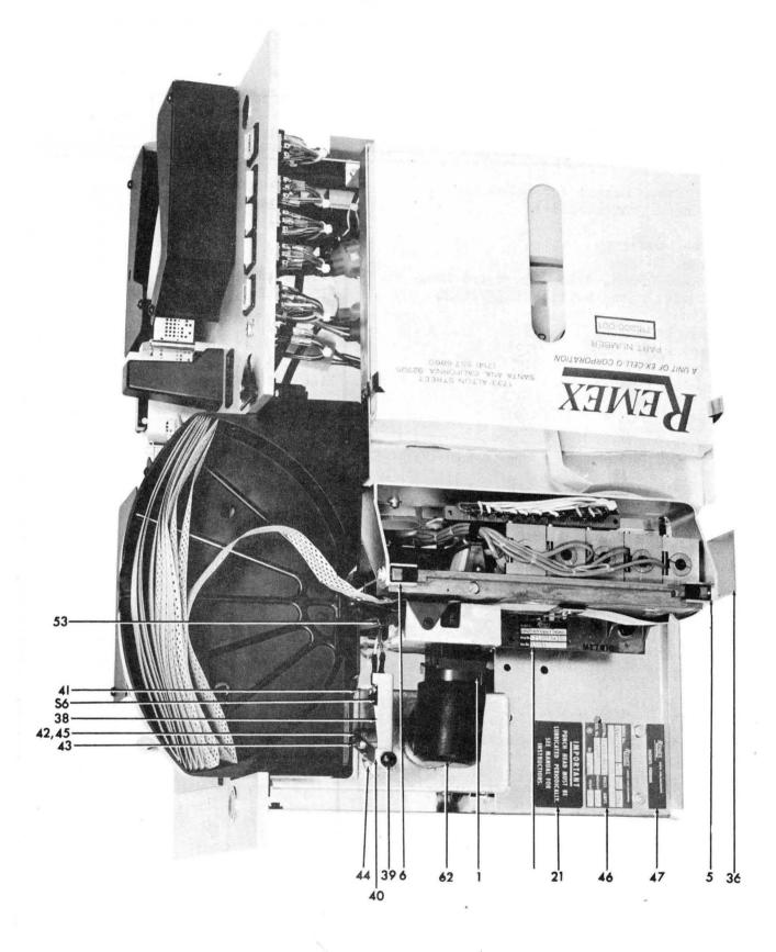
Figure 7-8. RAF3075BCX, Top View, Showing the Threading of the Tape
