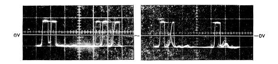
Two Examples of Anti-Jitter Control Misadjusted SCALE: 0.5 V/CM, 5 MSEC/CM
