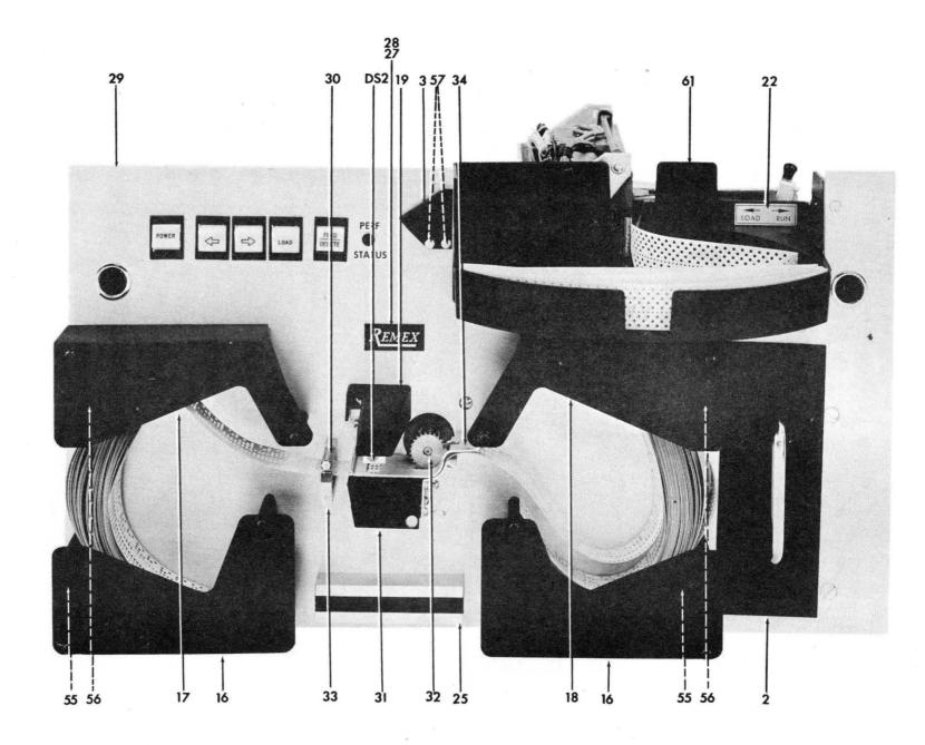
Figure 7-9. RAF3075BCX, Front View of Front Panel
