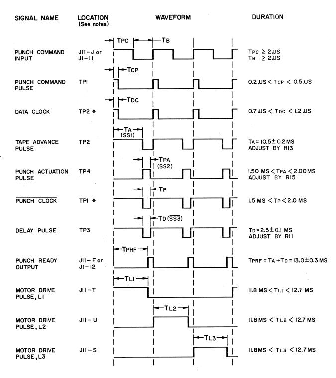
NOTES: I. ALL LOCATIONS EXCEPT (\*) ARE ON CONTROL LOGIC AND FEED HOLE DRIVER CARD. LOCATIONS MARKED WITH (\*) ARE ON DATA LOGIC AND DRIVER CARD ALTHOUGH THESE SIGNALS ARE GENERATED ON THE CONTROL LOGIC AND FEED HOLE DRIVER CARD.
