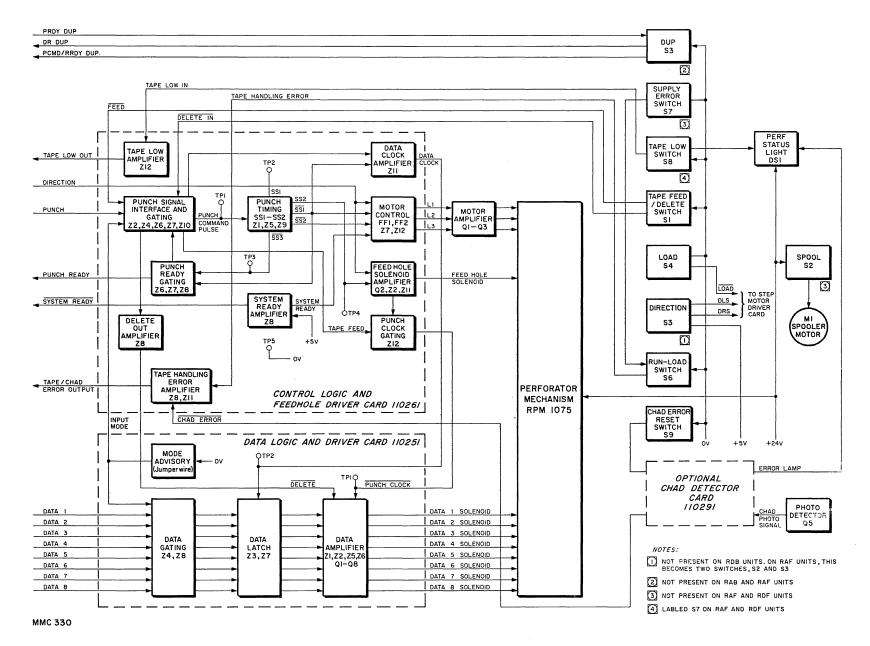
Figure 4-1. Block Diagram, Punch Control Section
