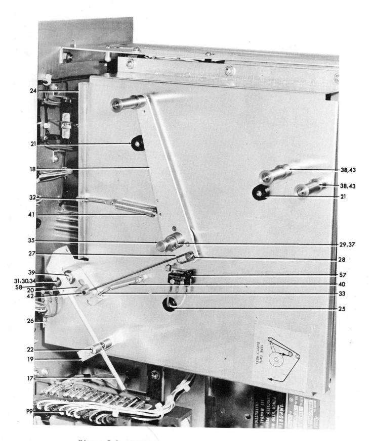
Figure 7-3. RDB3075BCX, Top View of Deck Assembly with Hub Assembly
