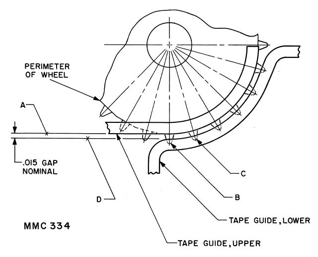
Figure 5-4. Setting of the Lower and Upper Tape Guides in Relation to the Sprocket
