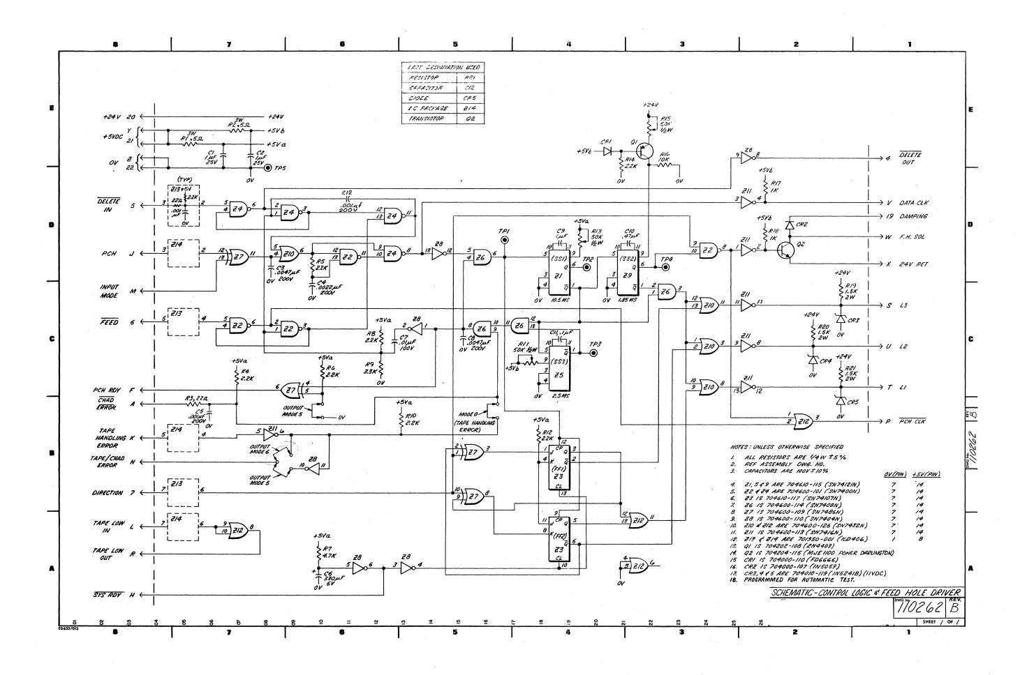
Figure 8-5. Schematic, Control Logic and Feed Hole Driver Card 8-11/8-12 RSM-207V 110261
