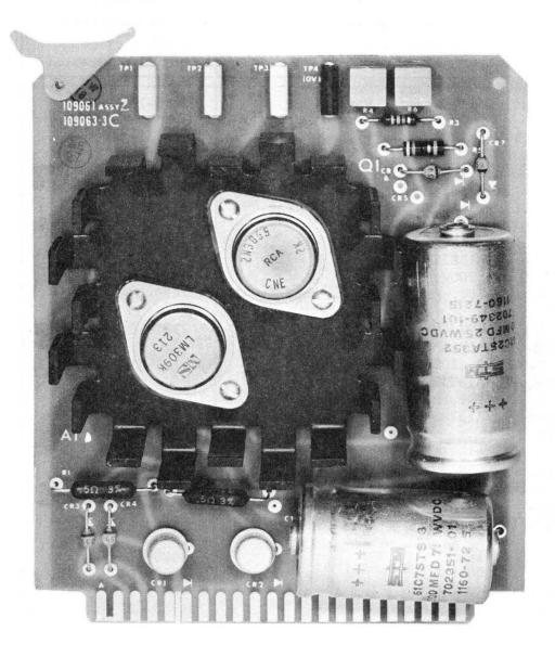
Figure 7-15. Step Motor Power Supply Card 109061-2 Assembly.
