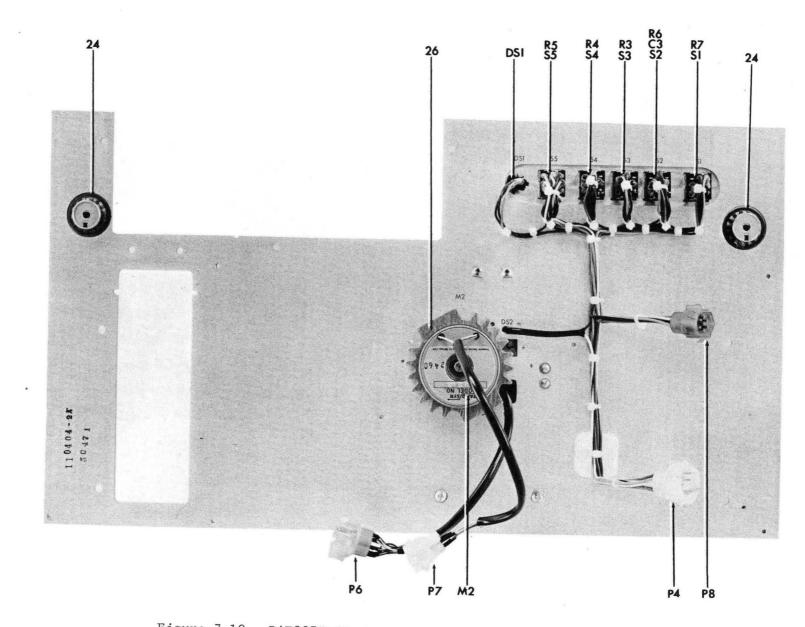
Figure 7-10. RAF3075BCX, Rear View of Front Panel
