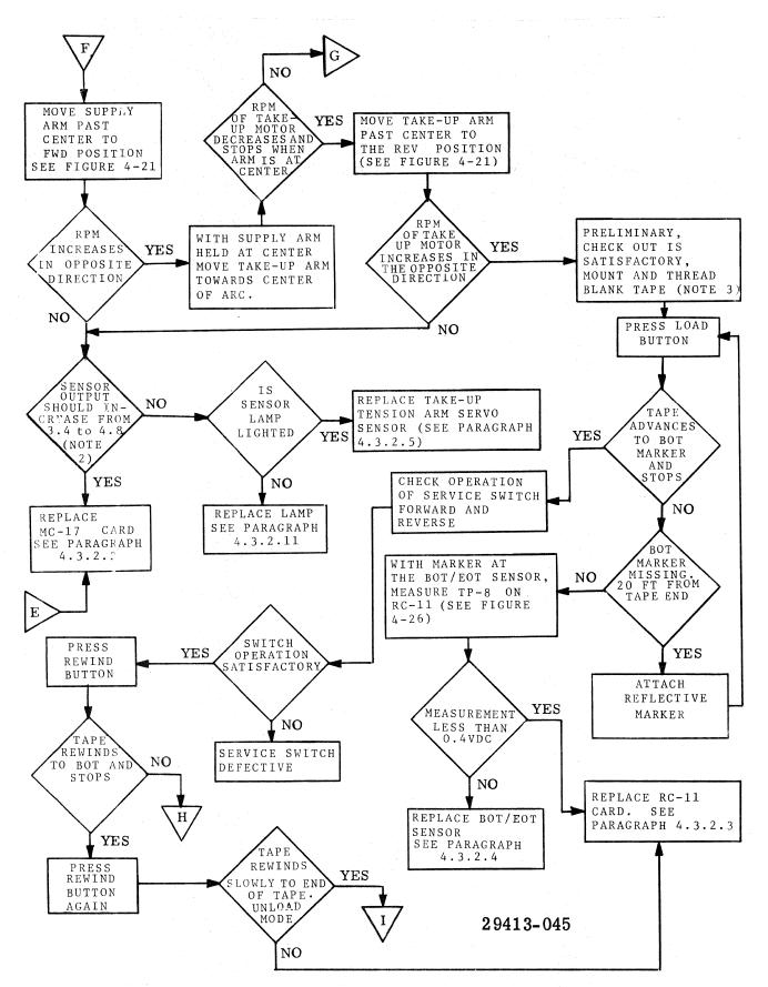
Figure 5-1. Troubleshooting Diagram, Preliminary Checkout, Load Sequence and Test Write/Read Sheet 3 of 4
