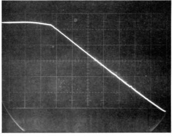
EXT. TRIGGER SLOPE (+) SWEEP: 2ms/cm VERT. GAIN: 0.2v/cm
