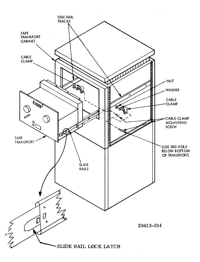
Figure 4-4. Tape Transport Slide Rail/Removal.
