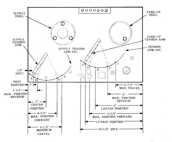
Figure 4-21. Location of Tension Arm Operating Positions.
