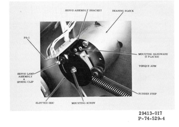
Figure 4-7. Tension Arm Servo Sensor Disassembly.
