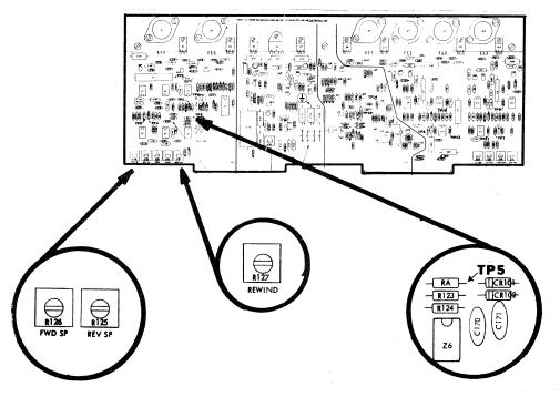
Figure 4-23. Forward Speed Adjustment/Test Point Location.
