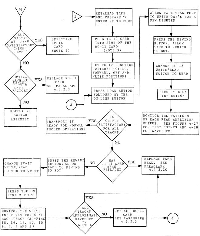
Figure 5-1. Troubleshooting Diagram, Preliminary Checkout, Load Sequence and Test Write/Read Sheet 4 of 4
