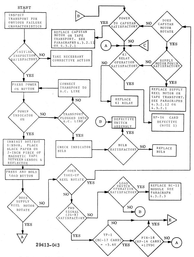
Figure 5-1. Troubleshooting Diagram, Preliminary Checkout, Load Sequence and Test Write/Read Sheet 1 of 4
