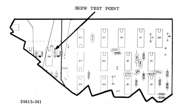
Figure 4-31. Read Skew Test Point.
