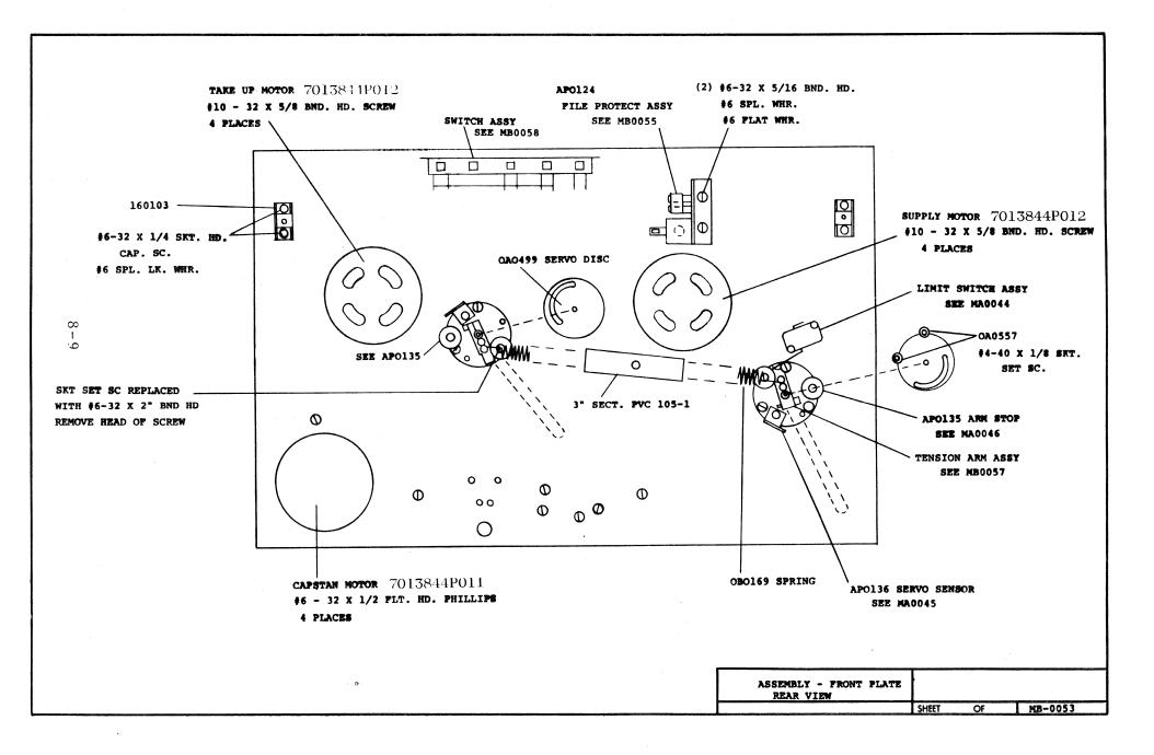
PART NO. ITEM QUANTITY DESCRIPTION ACTUATOR #4-40x1/8 SKT SET SCREW SENSING ROD #4-40x1/2 SKT SET SCREW 8-10 SOLENOID PLUNGER QA0466 SPRING SHOULDER WHR 5/16 SOLENOID . 8 #4-40x1" BND ND SCREW SWITCH STANDOFF FILE PROJECT BRACKET OB0144 #6 FLT WMR #6 SPL LK WHR #6-32x1/4 BHD HD SCREW #4 PLTWER #4 SPL LK WHR \$4-40 HEX NUT
