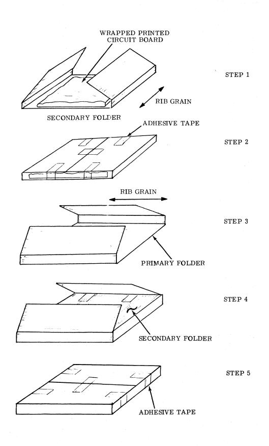
Figure 6-2. Printed Circuit Board Shipping Configuration.
