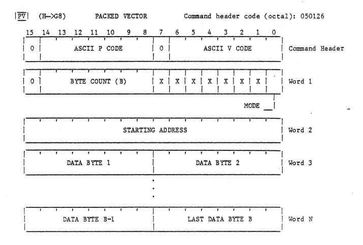
Bits 8 through 14 in word 1 contain the byte count indicating the number (B) of data bytes contained in the PV message. Bit 0 in word 1 selects the mode. When bit 0 is set to 0, add mode is selected. For add mode, an RTRN, return instruction is added to the end of the refresh code created from the data bytes contained in the PV message.
