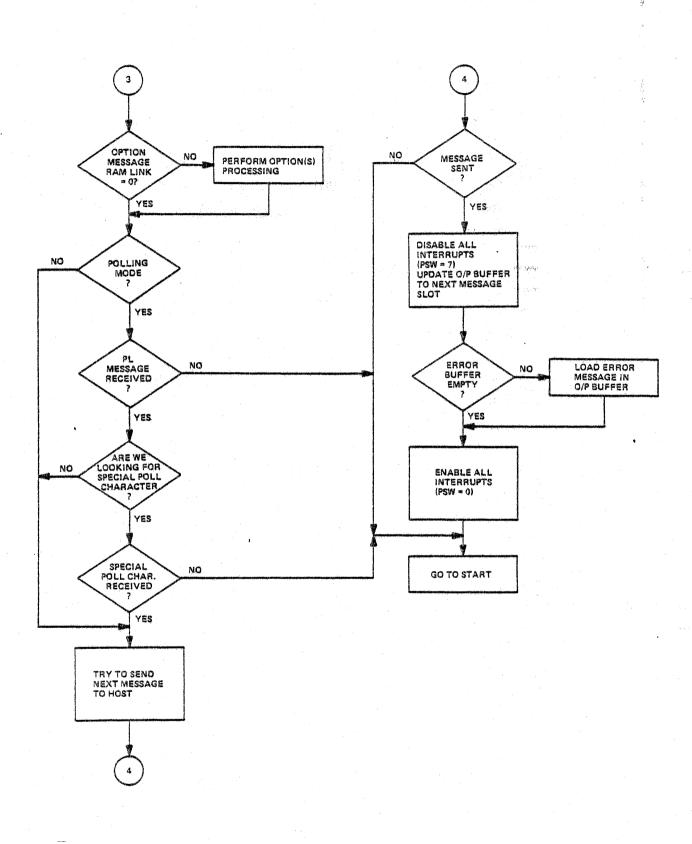
Figure 7-1. GCP Executive Loop Flowchart (Sheet 2 of 2)
