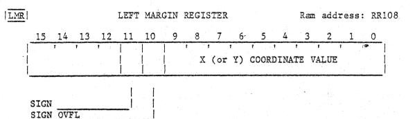
The left margin register contains the X position value (or Y position value if rotated text) that defines the position at which the next character will be presented whenever a CR control character is encountered. The margin value is stored when an STX character is specified in a CHAR or TXT instruction as the current DXR (or DYR).
