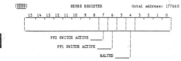
The sense register is a one-bit register that indicates the halt status of the digital graphic controller. The remaining bits are not used. The condition indicated by bit 4 when it is set to 1 is as follows:
