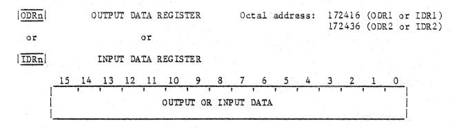
The data register is a dual-purpose register referred to as an output data register (ODRn) when data is being transferred from the host computer to the GRAPHIC 8 and as an input data register (IDRn) when data is being transferred from the GRAPHIC 8 to the host computer.
