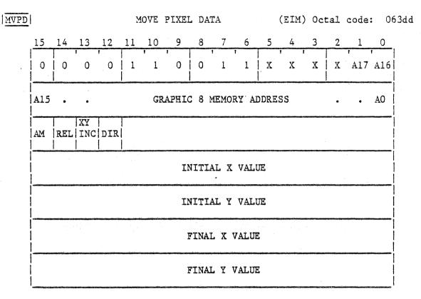
MVPD controls the transfer of data between the selected mapping (Pixel) memory and the display processor memory. The data is defined by the GRAPHIC 8 memory address (bits AO to A17). The Initial X and Y values and the Final X and Y values represent the rectangular array of pixels involved in the transfer.
