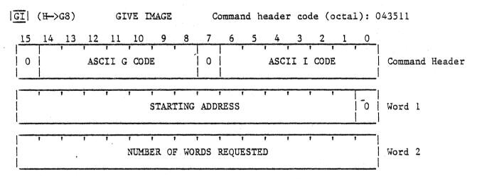
The GI message is a three-word message that causes GCP to send back to the host computer the contents of the GRAPHIC 8 memory beginning at the specified starting address and ending when the requested number of words have been sent. The specified starting address should be the address of an even-numbered byte. If, however, an odd address is specified, the low order bit is ignored by GCP and no XX (error status) message is generated.
