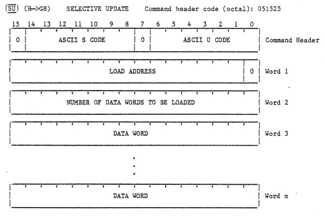
The SU message is a variable-length message that operates in exactly the same manner as the MU (memory update) message except that the digital graphic controller is not halted. Therefore, if an SU message is used to update a refresh file currently being processed by the graphic controller, the file must remain valid as each data word is replaced.
