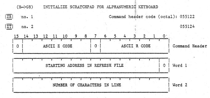
This three word Initialize Scratchpad message is used to establish parameters for handling alphanumeric characters on a line basis from the keyboard. It is used in conjunction with a refresh file that contains an area reserved for storage of characters typed in by the operator. This area, called a scratchpad, typically consists of a sequence of TXT (draw two tabular characters) instructions with ASCII codes for spaces.
