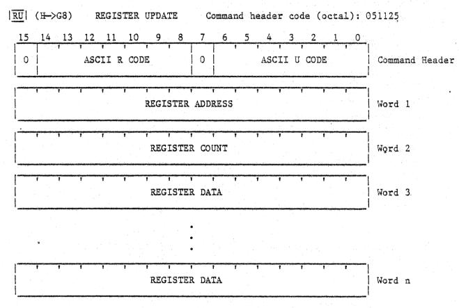
. The RU message is a variable length message that is used to update a series of registers in the I/O address area of the hardware. Word 1 contains the address of the first register to be updated. Valid register addresses are in the range of 160000-177777 (octal). Word 2 contains the register count indicating the number of successive registers to be updated. Words 3 through n contain the data values to be loaded into each register.
