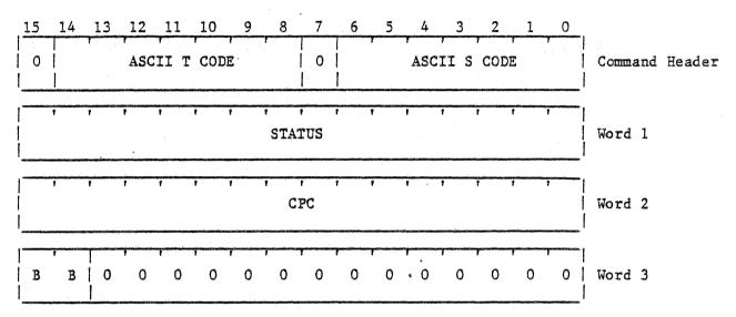
The 2-D/3-D coordinate converter can generate 16 interrupt conditions, provided that the corresponding mask bits are enabled. The TS message is returned to the host computer when a 3D coordinate converter interrupt condition occurs.
