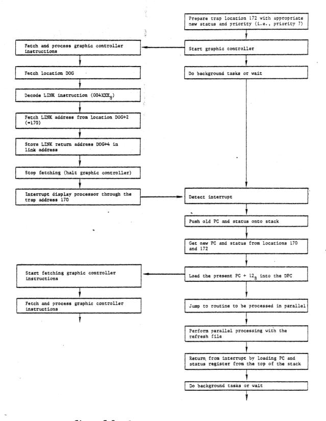
Figure 7-7. Super Sync Flow Chart Example
