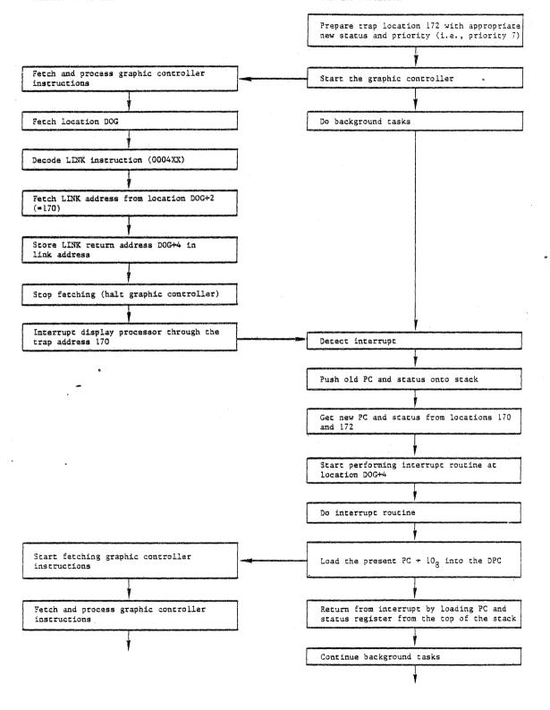
Figure 7-5. Sync Link Flow Chart Example
