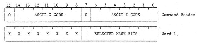
The ZI message is a two word message used to selectively disable mask register (MKR) associated interrupts. If a mask bit is set to 1, then the interrupt associated with that bit is disabled. If a mask bit is set to 0, then the interrupt associated with that bit remains unchanged after the ZI message is processed by GCP.
