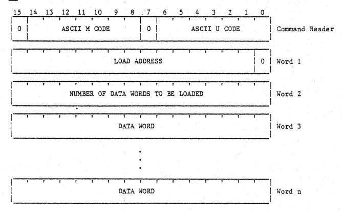
The MU message is a variable-length message used to load data into the read/write memory of the GRAPHIC 8. The load address specified in word 1 tells GCP the address at which loading of the data should begin. This address must be the address of an even-numbered byte. An odd address will result in an XX (error status) message being returned by the GRAPHIC 8 and data will not be loaded.
