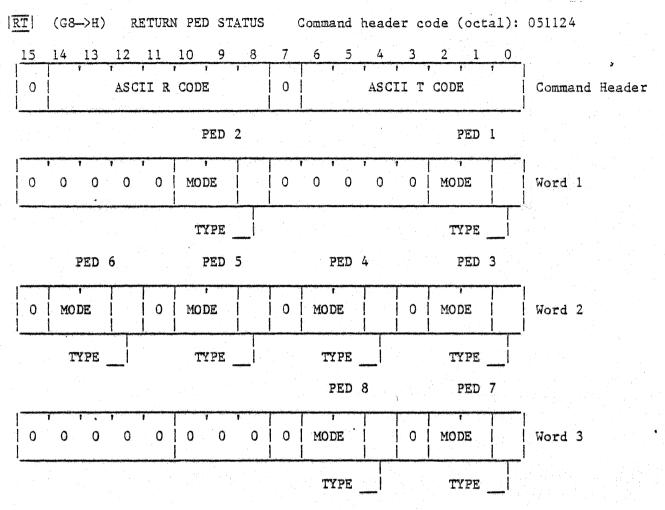
The RT message is sent by GCP to the host computer in response to a GS message. Word 1 contains the software status of each PED.
