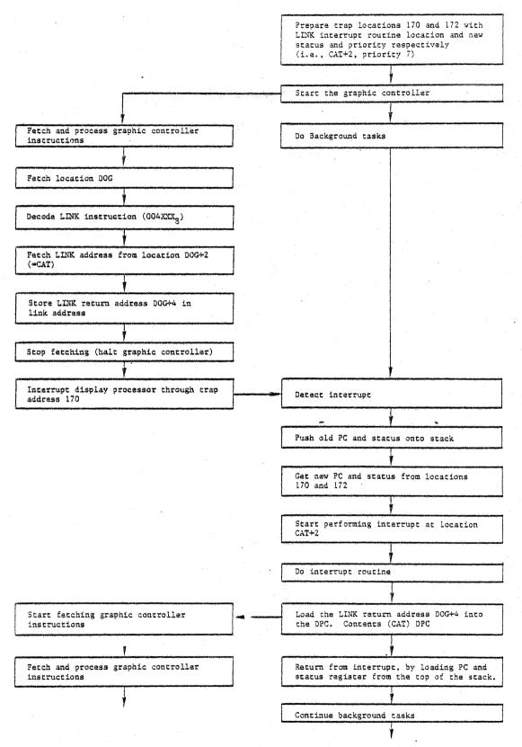
Figure 7-3. Synchronized Linkage Flow Chart Example
