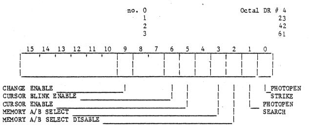
The Video Controller Status register contains data that controls the presentation of screen data.
