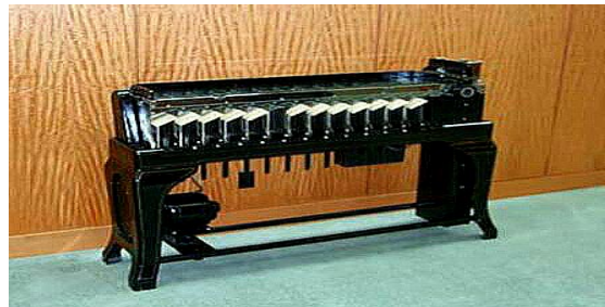
Punched card sorting machine
