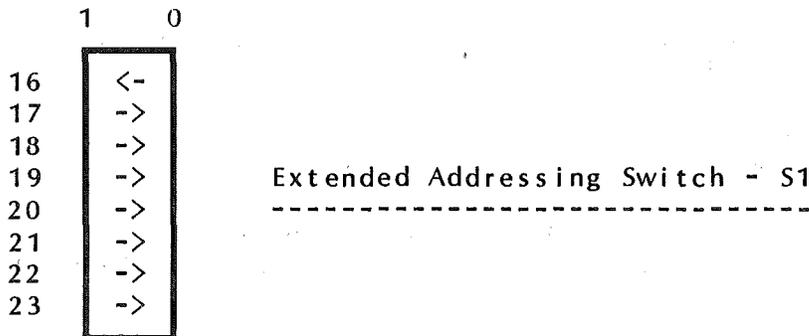
Processors such as the 8086, which provide twenty significant address lines, usually drive A20 - A23 low. The switch positions corresponding to A20 - A23 should be set to the "0" position for these processors.
