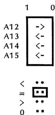
Example: 48K memory board which resides between 0 and BFFF hex. In this example we wish to disable everything above the 4K block at B000 hex. Set the address to B hex as follows, A12 = 1, A13 = 1, A14 = 0, A15 = 1. Put the shunt on the pair of pins to the right of the ">".
