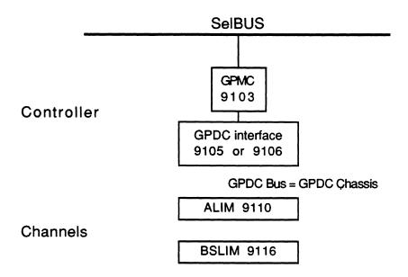
Refer to the GPMC Technical Manual, 325-329104/9103 for details of the GPMC operation. Refer to the appropriate technical manual part number 325-32xxxx, where xxxx is the model number, for details of a particular GPDC channels operation.
