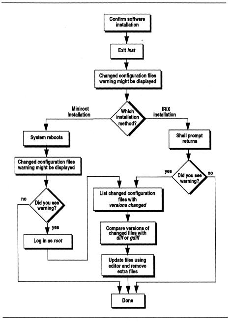
Figure 6-1 Finishing Up Installation Flowchart
