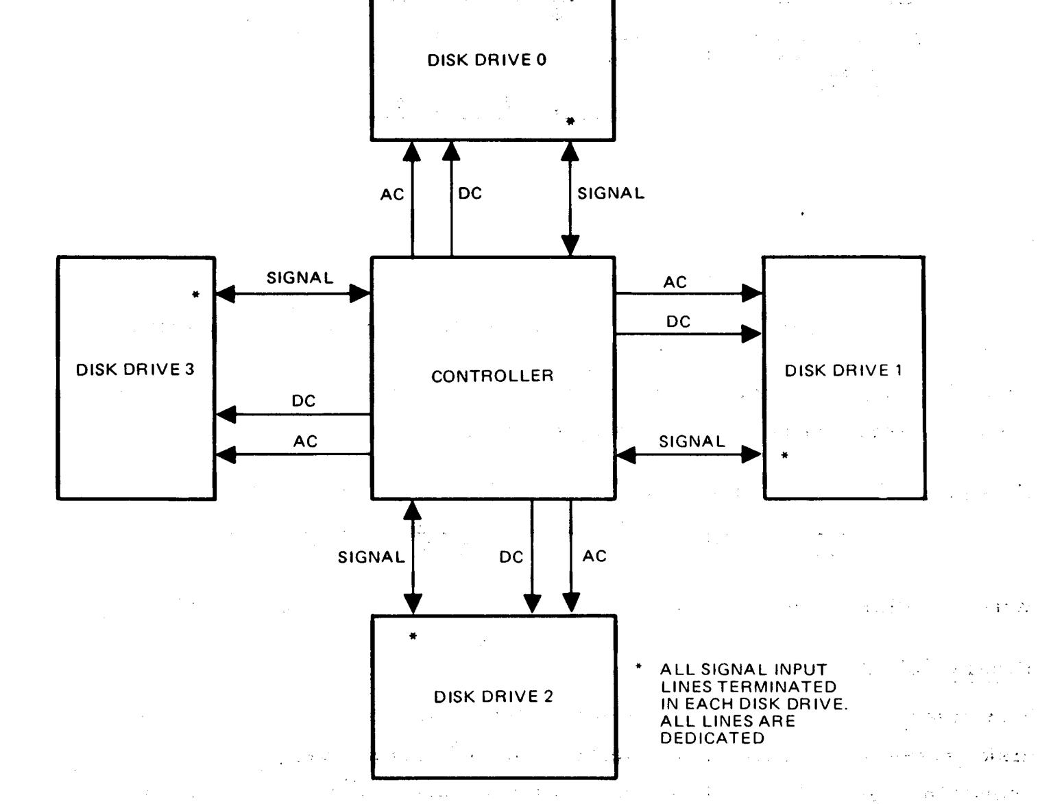
Figure 4-6. Radial Select Configuration
