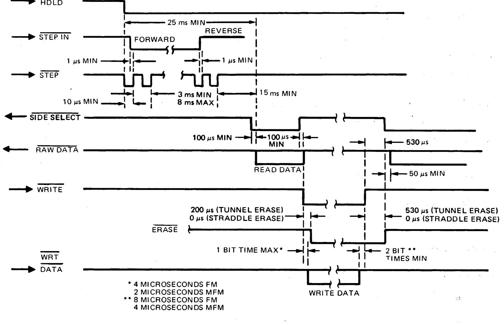
Figure 3-6. Control and Data Timing
