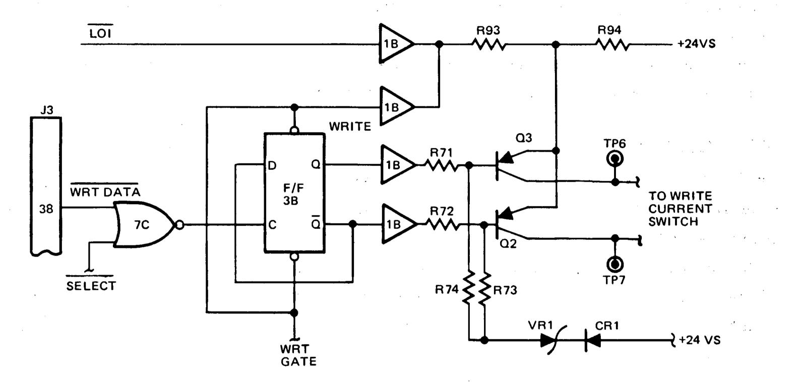
Figure 3-27. Write Current Control Logic
