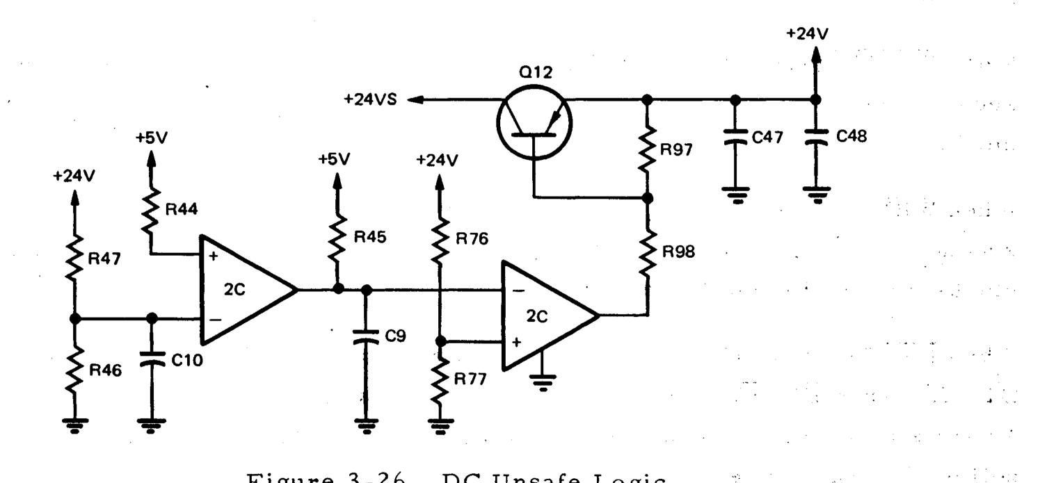
Figure 3-26. DC Unsafe Logic
