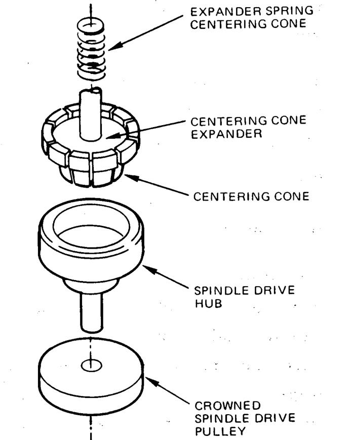
Figure 3-4. Spindle System
