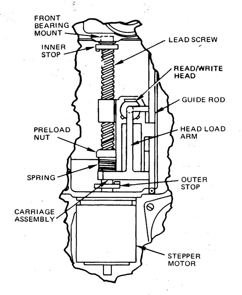
The read/write head carriage rides on the lead screw shaft and is held in horizontal alignment. When the stepper motor is pulsed, the lead screw rotates clockwise or counterclockwise, moving the carriage in or out, respectively
