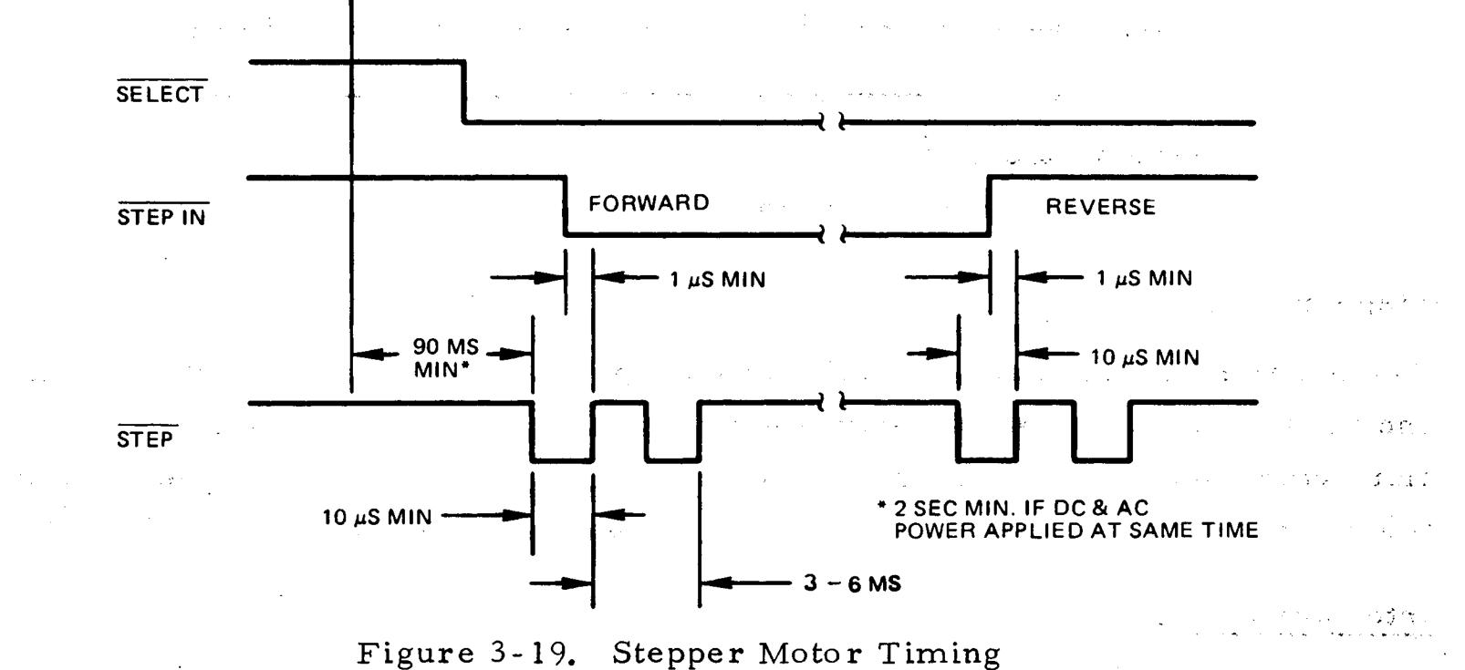
When STEP IN becomes active, the counter is set to the forward mode. State Counter
