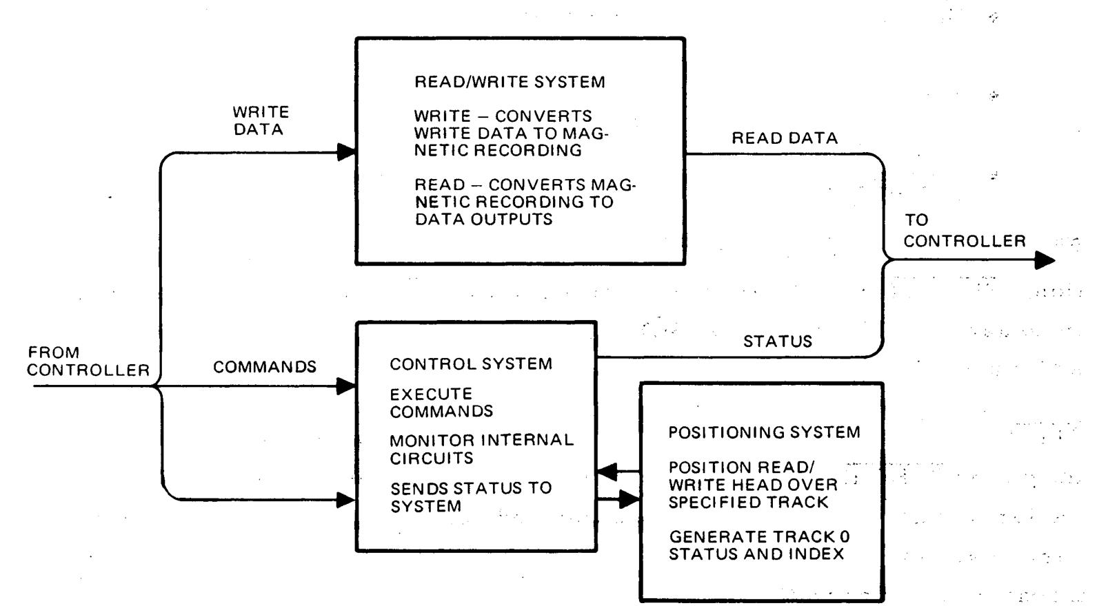
Figure 3-1. Floppy Disk Drive. Simplified Block Diagram
