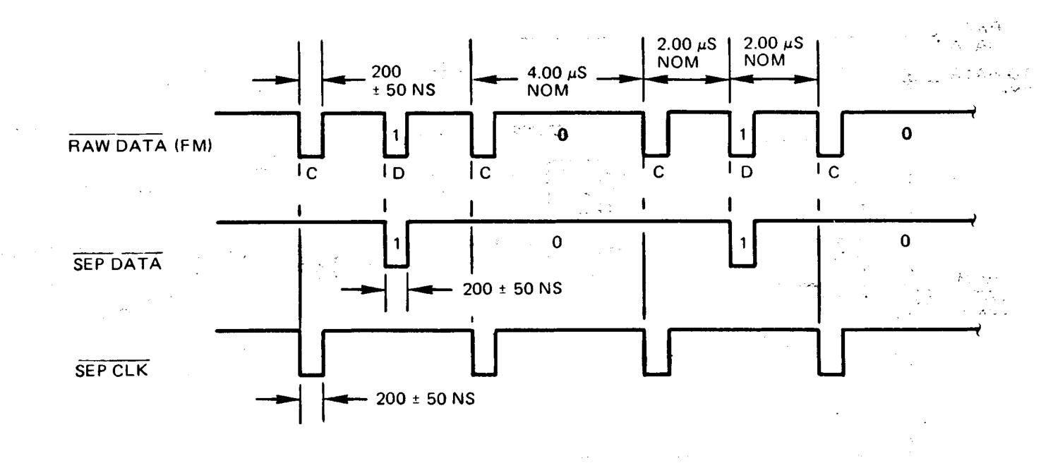
Figure 3-38. FM Data Separator Output Timing
