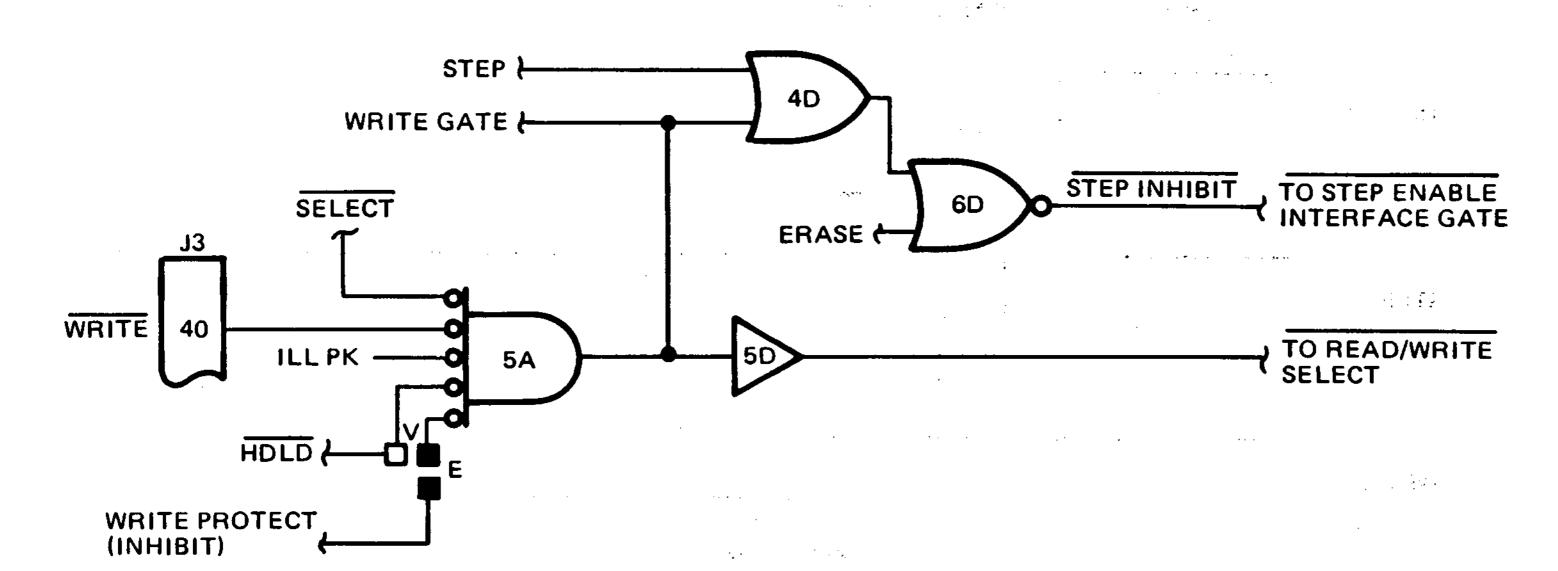
Figure 3-23. Write and Erase Gating Logic
