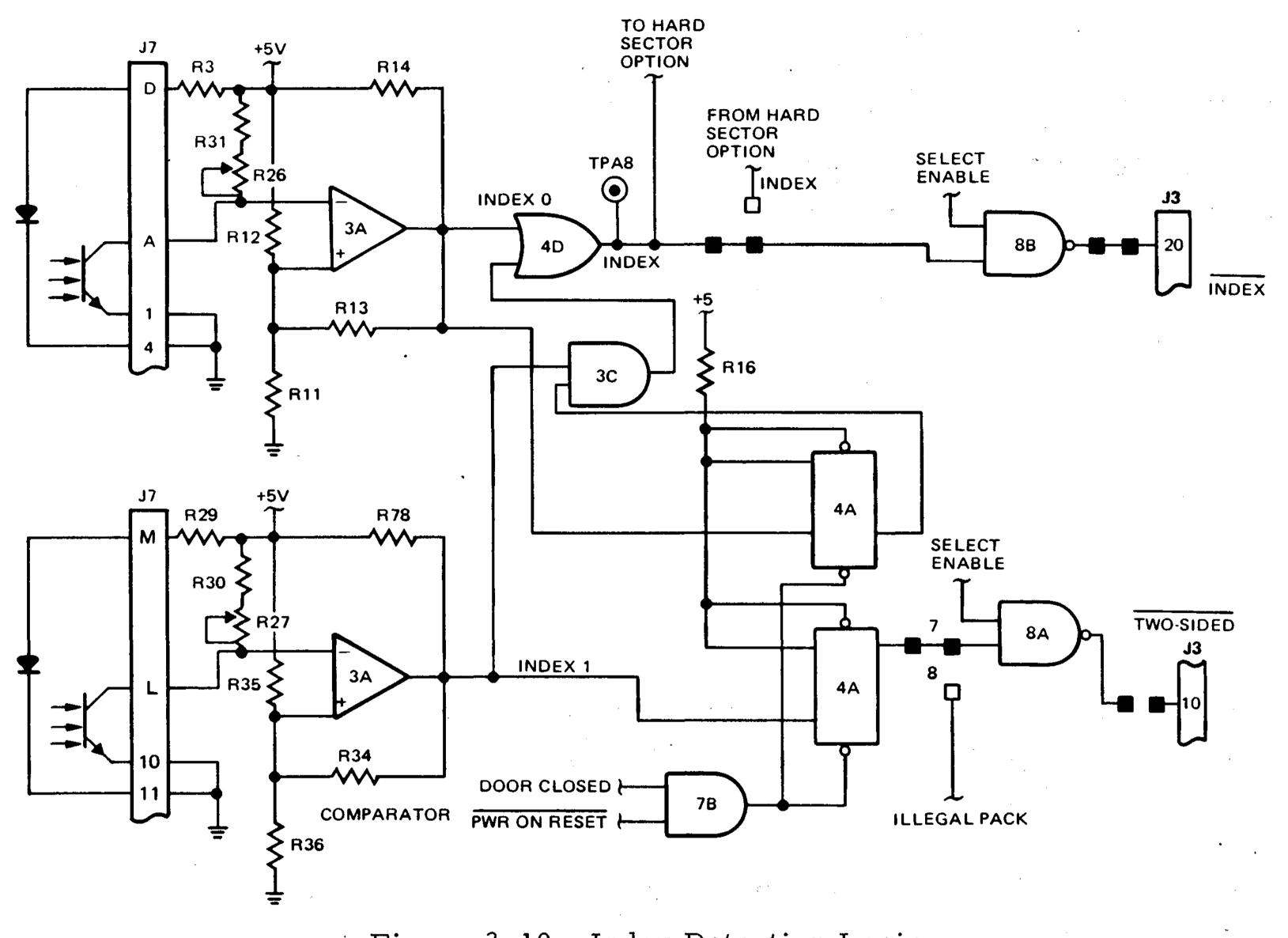
Figure 3-10. Index Detection Logic
