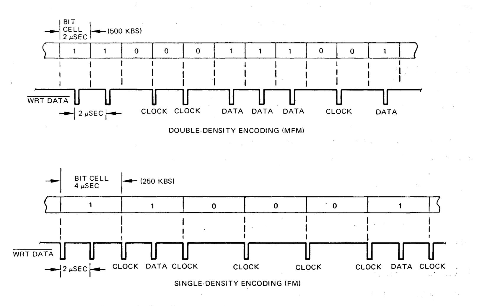
Figure 1-3. Single and Double Density Encoding
