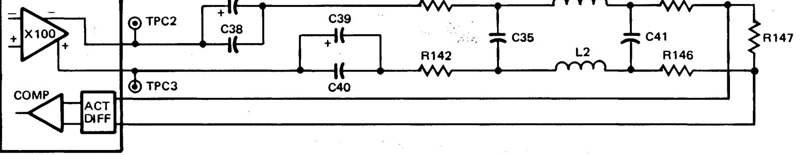
Figure 3-33. Read Preamplifier and Filter Circuit
