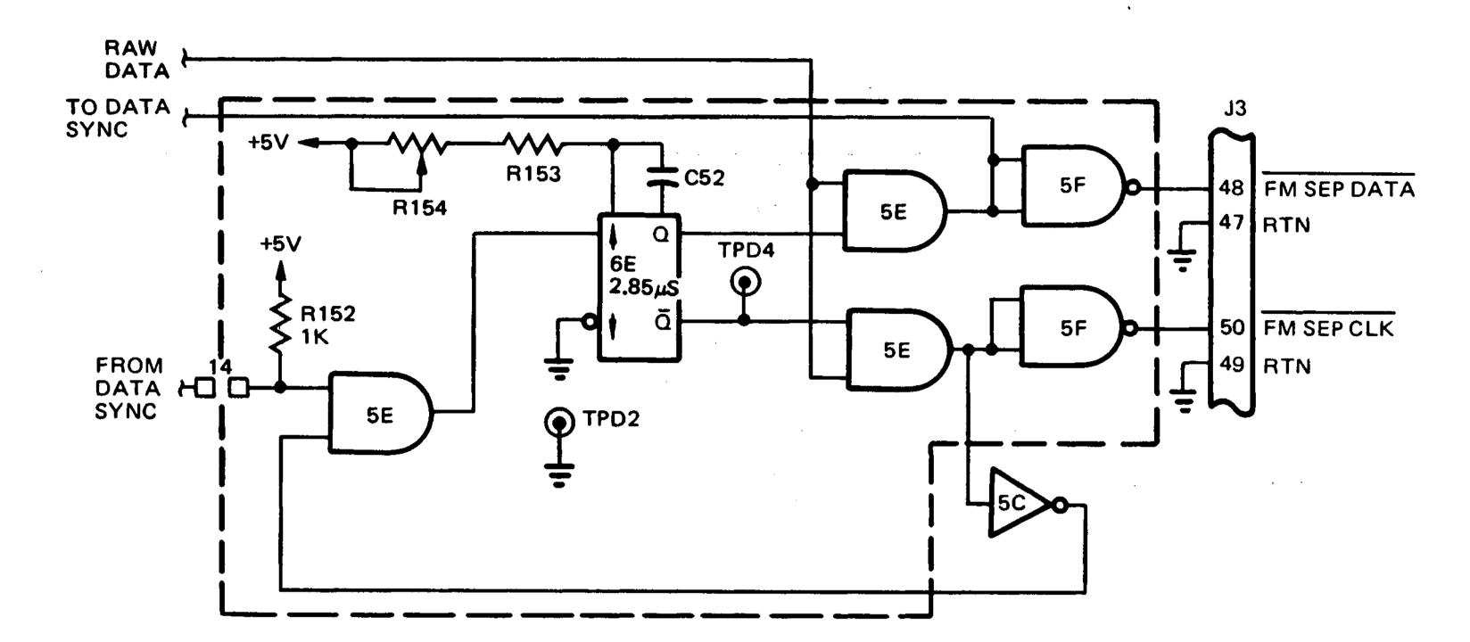
Figure 3-37. FM Data Separator (Option) Logic
