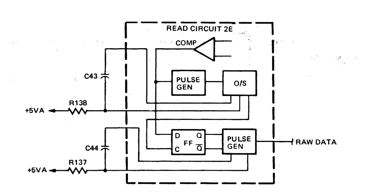
Figure 3-36. Time Domain Filter Logic
