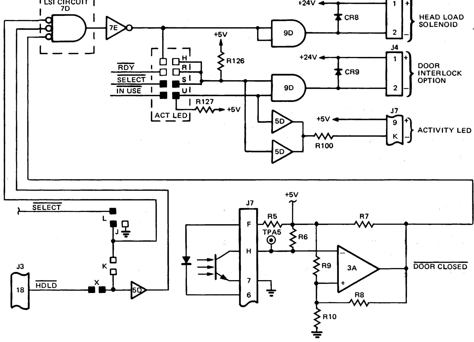
Figure 3-15. Head Load Logic
